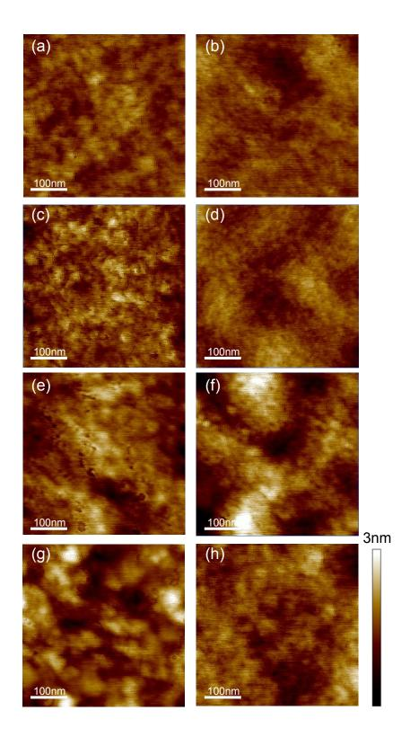
FIG. S2. AFM images of the P3HT:PCBM blends: (a) and (b)  $p_{P3HT} = 0.41$ , (c) and (d)  $p_{P3HT} = 0.51$ , (e) and (f)  $p_{P3HT} = 0.63$ , (g) and (h)  $p_{P3HT} = 0.85$ ; with thermal treatments: left column (a) – (g) corresponds to heterogeneous active layers, while right column (b) – (h) corresponds to homogeneous active layers.
