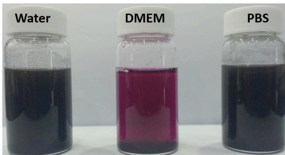
**Figure S9.** The CB[6]-MNPs can be easily dispersed in water, cell culture medium (DMEM) and phosphate buffer solution (PBS) to form a stable dispersion that can stand for more than two days without visible sedimentation.
