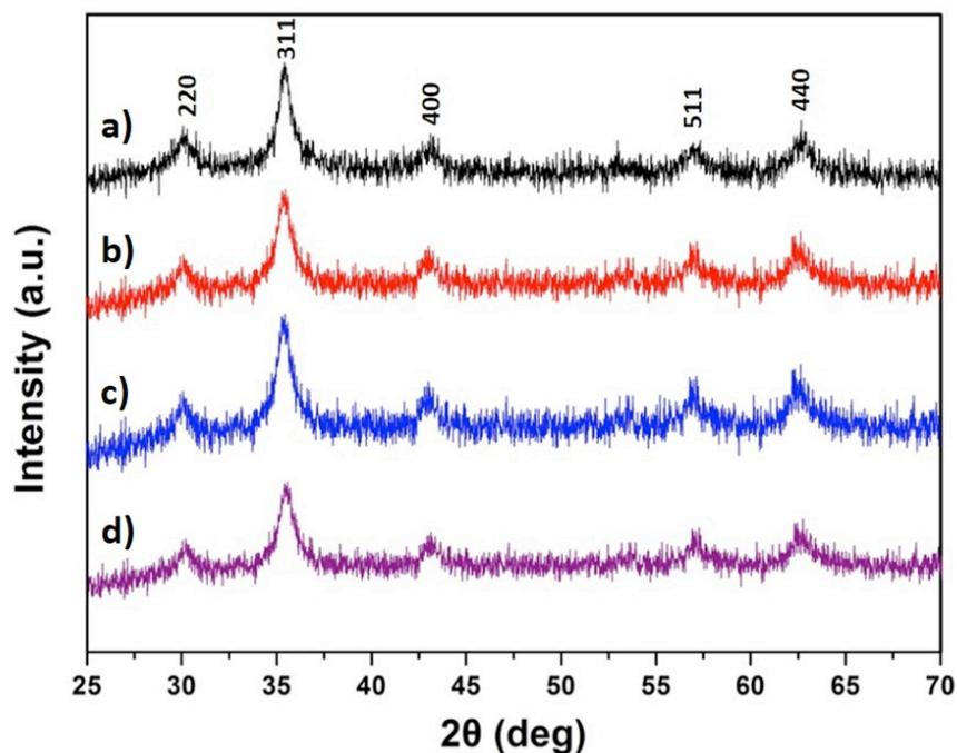
**Figure S5.** XRD patterns of CB[6]-MNPs obtained with different reaction time of a) 12 h, b) 10 h, c) 8 h, and d) 6 h.
