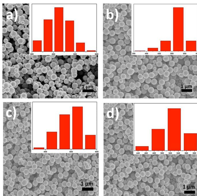
**Figure S2.** The SEM images and size distributions of CB[6]-MNPs synthesized by the typical solvothermal reaction with  $\text{FeCl}_3$  (4.0 mmol), CB[6] (0.2 mmol), and NaAc (14.6 mmol) in ethylene glycol (20 mL) at 200 °C for different reaction time: a) 6 h, b) 8 h, c) 10 h, and d) 12 h.
