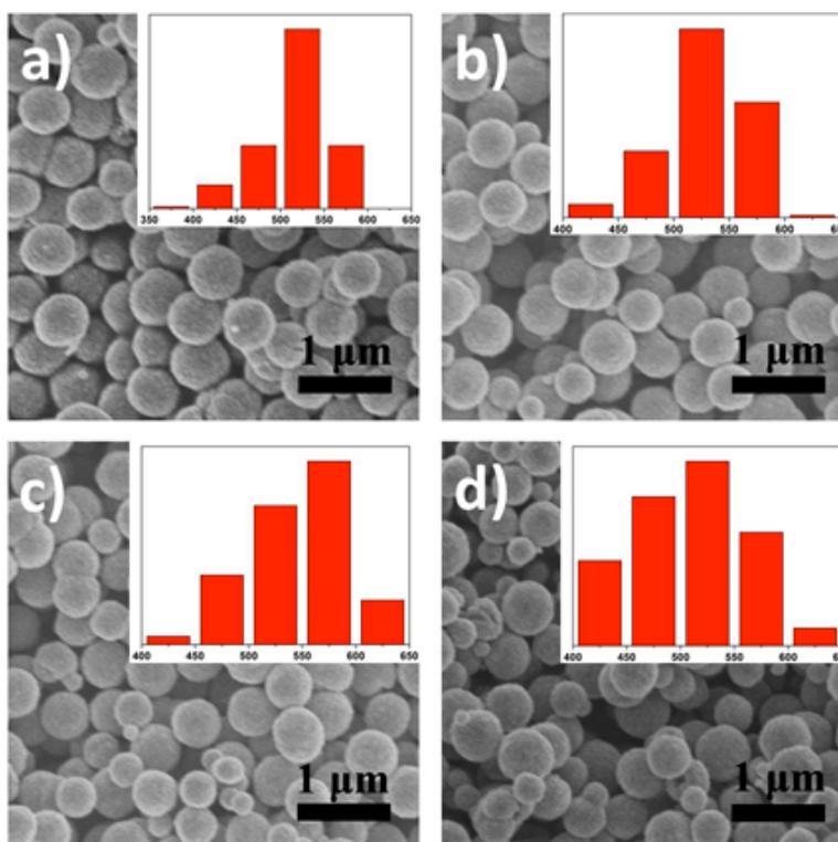
**Figure S1.** The SEM images and size distributions of CB[6]-MNPs synthesized by the typical solvothermal reaction with FeCl<sub>3</sub> (4.0 mmol), CB[6] (0.2 mmol), and NaAc (14.6mmol) in ethylene glycol (20 mL) for 10 h, and maintained at a) 200 °C, b) 210 °C, c) 220°C, and d) 230 °C.
