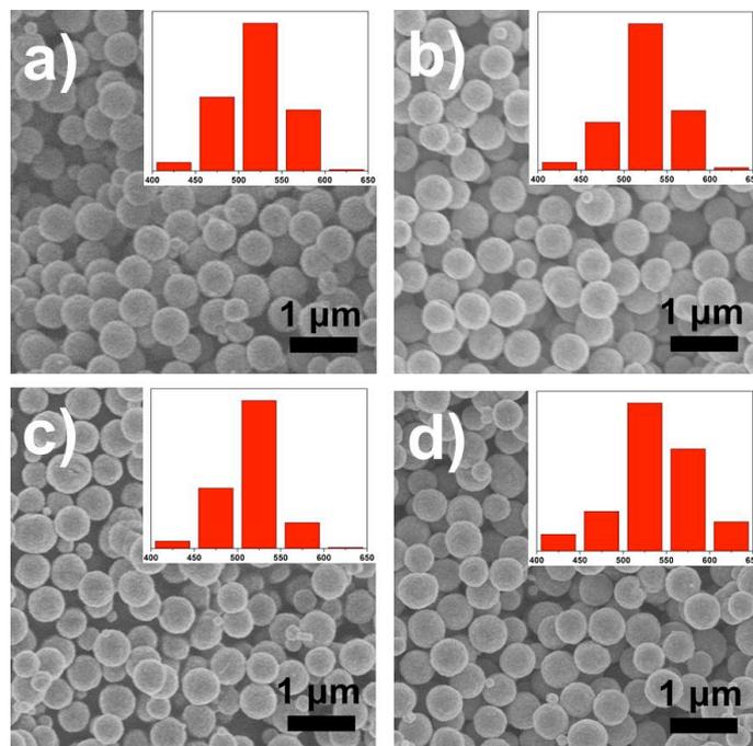
**Figure S3.** The SEM images and size distributions of CB[n]-MNPs: a) CB[5]-MNPs, b) CB[6]-MNPs, c) CB[7]-MNPs, and d) CB[8]-MNPs, synthesized by the typical solvothermal reaction with  $\text{FeCl}_3$  (4.0 mmol), CB[n] ( $n = 5-8$ , 0.2 mmol), and NaAc (14.6 mmol) in ethylene glycol (20 mL) at 200 °C for 10 h.
