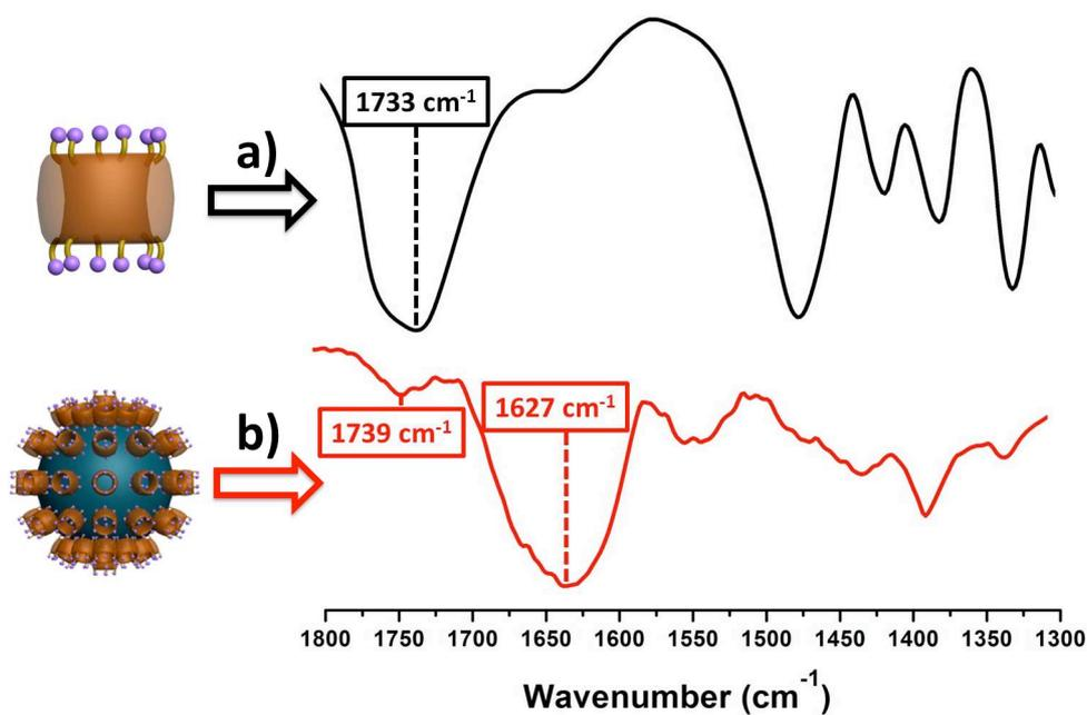
**Figure S6.** Selected area of FT-IR spectra of bared CB[6] (a) and CB[6]-MNPs (b), showing the changes of carbonyl absorption bands.
