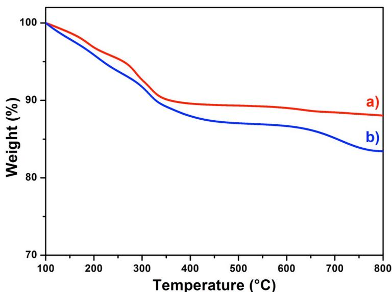
**Figure S10.** TGA curves of a) bare Fe<sub>3</sub>O<sub>4</sub> MNPs without CB[n] modification; b) CB[6]-MNPs. TGA curves were obtained at nitrogen atmosphere with a heating rate of 10 K min<sup>-1</sup>.
