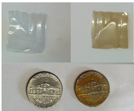
Figure SI-1 . TOP: pDA and pCDA thin films on glass coverslips produced by oxidation of 10 mM DA and CDA for 8h. BOTTOM: pCDA films on cuttings from polyethyleneterephthalate (PET) bottles and metals (right) as obtained by dip-coating into CDA at 10 mM in for 24 h, against controls (left)
