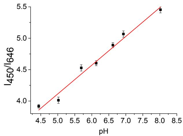
Fig. S1 The luminescence intensity ratio ( $I_{450\text{nm}}/I_{646\text{nm}}$ ) of UCNPs@SiO<sub>2</sub>-XO as a function of pH value. Solid line represents fit with a correlation coefficient of 0.99.
