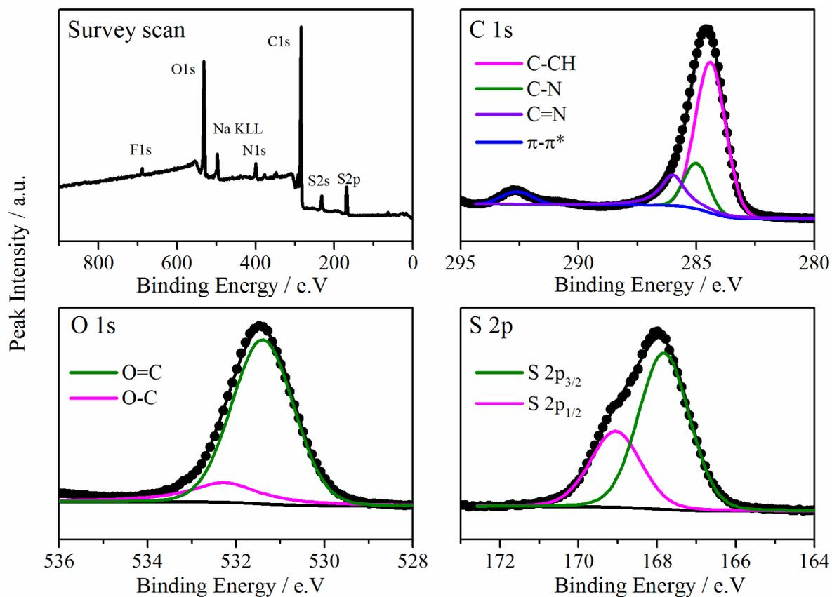
**Fig. S1:** An example of survey spectra and high resolution fitted curve of elements of *p*TSA-doped PANI film at fabrication. C 1s has been fitted to have C-CH, C-N, C=N and  $\pi-\pi^*$ . O 1s spectra fitted to have O=C and O-C. S 2p spectra shows spin doublet which are S 2p<sub>3/2</sub> and S 2p<sub>1/2</sub>.
