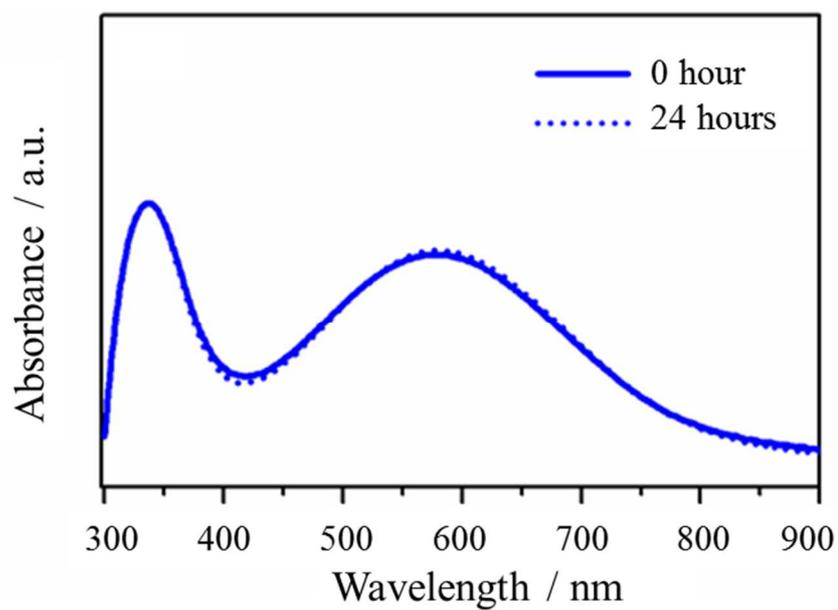
**Fig. S3:** UV-Vis spectra of undoped PANI. The spectra shows two main absorption peaks indicating benzoid and quinoid segments at 345 nm and 592 nm, respectively. Post incubation in PBS, no changes of the absorption spectra of PANI observed.
