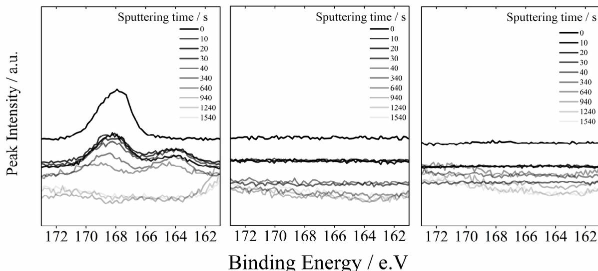
**Fig S2:** Depth analysis of S 2p signal with respect to Ar<sup>+</sup> sputtering time for (A) *p*TSA and (B) CSA-doped PANI at fabrication and following incubation in PBS for 0.5 hour and 24 hours.
