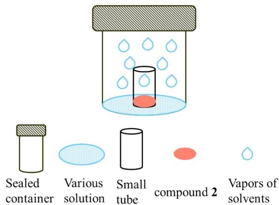
**Figure S6** Diagram of sensing measurements for different solvent-vapors.
