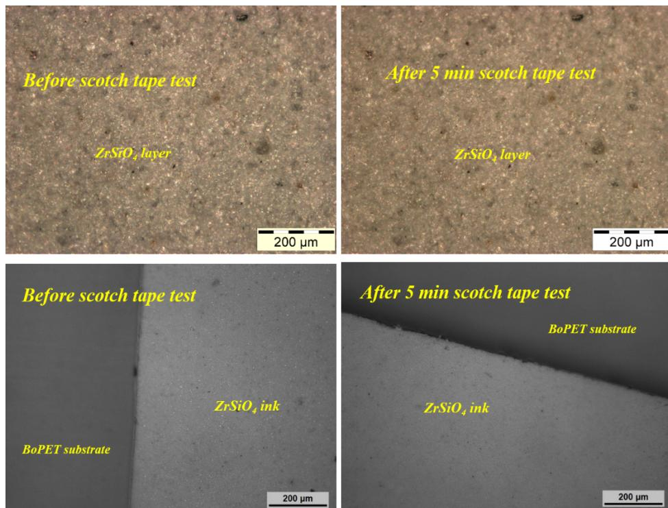
**Figure S1.** Optical microscopic images of surface and interface of  $ZrSiO_4$  layer before and after scotch tape test analysis.
