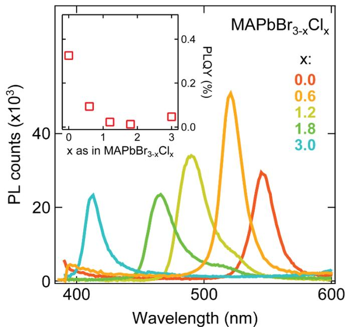
**Figure S5.** Raw photoluminescence spectra of MAPbBr<sub>3-x</sub>Cl<sub>x</sub> films. Inset: corresponding photoluminescence quantum efficiency (PLQY), expressed in percentage of emitted over absorbed photons.
