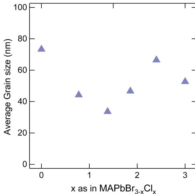
**Figure S2.** Average grain size of MAPbBr<sub>3-x</sub>Cl<sub>x</sub> films as determined from the analysis of XRD peak broadening. These values are representative of the shortest average grain dimension, and are consistent with the average grain height as determined from SEM (Figure S1).
