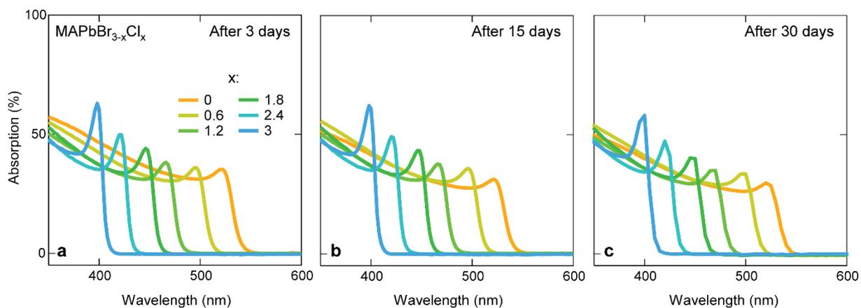
**Figure S4.** Optical absorption of MAPbBr<sub>3-x</sub>Cl<sub>x</sub> films measured over time after a) 3 days, b) 15 days, and c) 30 days from the day of fabrication.
