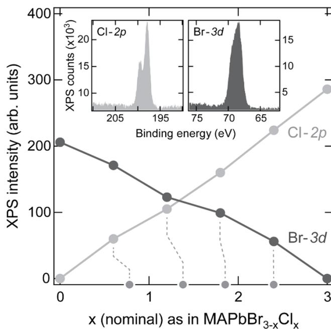
**Figure S3.** Plot of the Br and Cl XPS intensity (integrated area of the core-level peaks shown in the insets) as a function of nominal Br:Cl concentration (determined from the ratio of precursor molar mass). The Br:Cl ratio of XPS intensities, here used as a measure of the relative halide concentration, is represented by grey markers on the horizontal axis, with dashed lines highlighting the deviation from the nominal value.
