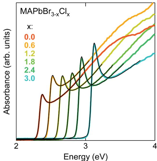
**Figure S6.** Optical absorption of MAPbBr<sub>3-x</sub>Cl<sub>x</sub> films (colored traces) and corresponding fit (black thin lines) combining the excitonic contribution (Equation 1) and the particle-hole continuum (Equation 2).
