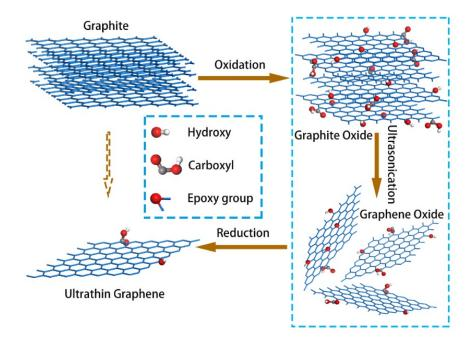
Fig. S1<sup>†</sup> Illustration for fabrication of graphene
