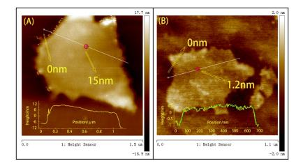
Fig. S3<sup>†</sup> AFM images of the (A) graphite and (B) graphene oxide.
