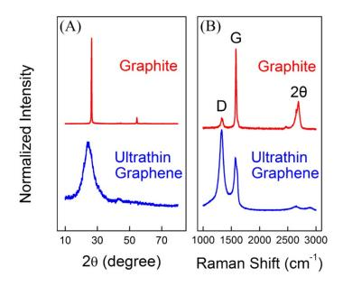
Fig. S2<sup>†</sup> XRD and Raman patterns of the graphite and ultrathin graphene, (A) XRD, (B) Raman spectrum.
