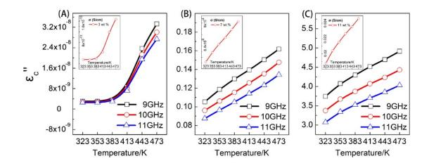
Fig. S4<sup>†</sup> The imaginary permittivity contributed by conductivity of the (A) 3 wt.%, (B) 7 wt.% and (C) 11 wt.% composites versus selected temperatures (323, 353, 383, 413 443 and 473K) at 9 GHz, 10 GHz and 11 GHz. The three insets are fitted conductivity of the (A) 3 wt.%, (B) 7 wt.% and (C) 11 wt.% composites versus selected temperatures (323, 353, 383, 413 443 and 473K).
