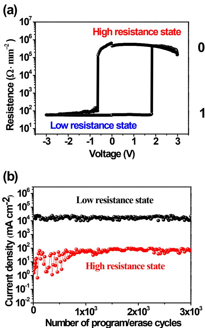
**Fig. S3** Additional characterization of the memristive device. (a) Resistance-Voltage characteristics of the memristor device: ITO/PEDOT:PSS/ $\text{CH}_3\text{NH}_3\text{PbI}_3$ /Cu. (b) Endurance performance of ITO/PEDOT:PSS/ $\text{CH}_3\text{NH}_3\text{PbI}_3$ /Cu memristor device.
