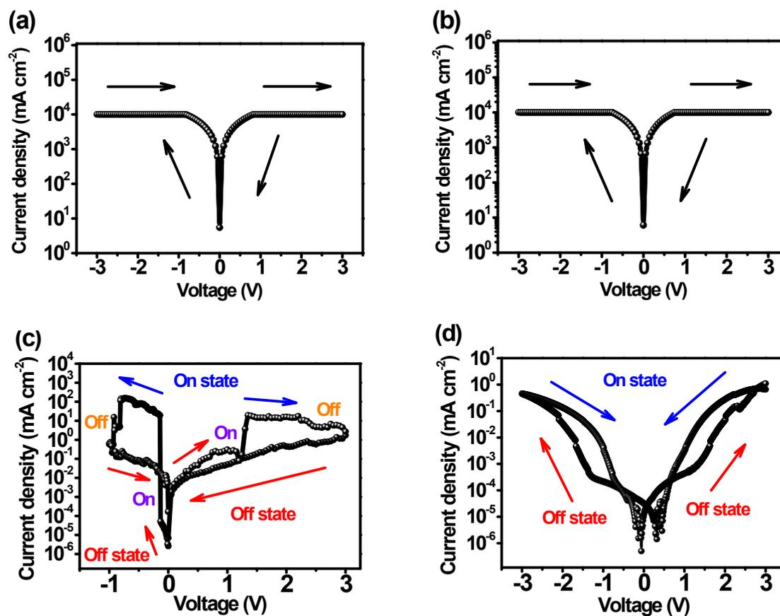
**Fig. S4** Current-Voltage ( $I$ - $V$ ) characterization of the control devices. (a) Cu/CH<sub>3</sub>NH<sub>3</sub>PbI<sub>3</sub>/Cu. (b) Cu/CH<sub>3</sub>NH<sub>3</sub>PbI<sub>3</sub>/Au. (c) ITO/PEDOT:PSS/CH<sub>3</sub>NH<sub>3</sub>PbI<sub>3</sub>/ITO. (d) ITO/PEDOT:PSS/CH<sub>3</sub>NH<sub>3</sub>PbI<sub>3</sub>/Au
