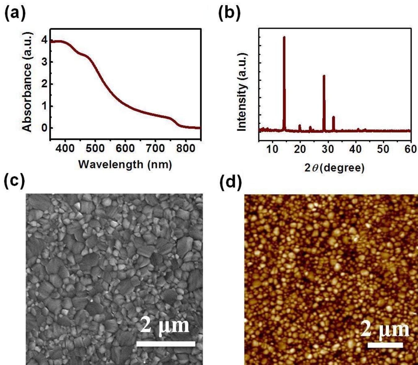
**Fig. S1** Organic-Inorganic hybrid perovskite characterization. (a) UV-Vis absorbance of  $\text{CH}_3\text{NH}_3\text{PbI}_3$  thin film on quartz. (b) X-Ray diffraction (XRD) spectrum of the perovskite material without Cu top electrode. (c) Scanning Electronic Microscope (SEM) image of the solution-processed perovskite film. (d) Atomic Force Microscope (AFM) image of the synthesized perovskite film.
