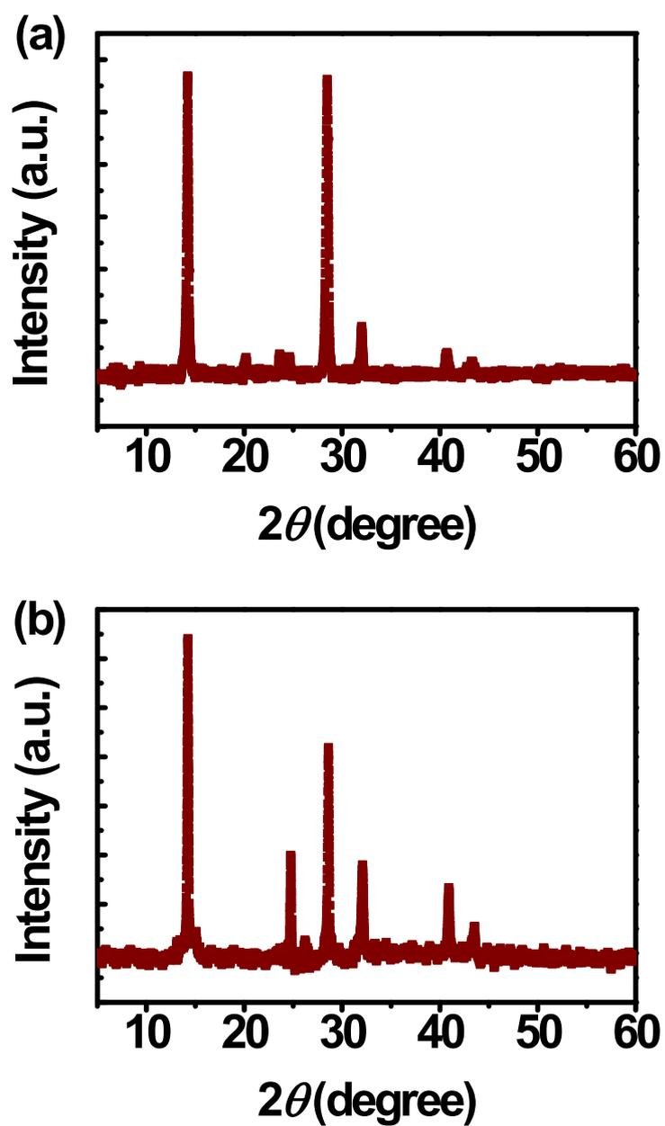
Fig. S5 X-Ray diffraction (XRD) spectra of (a)  $\text{CH}_3\text{NH}_3\text{PbI}_{3-x}\text{Cl}_x$ ; (b)  $\text{CH}_3\text{NH}_3\text{Pb}_{0.5}\text{Sn}_{0.5}\text{I}_3$ .
