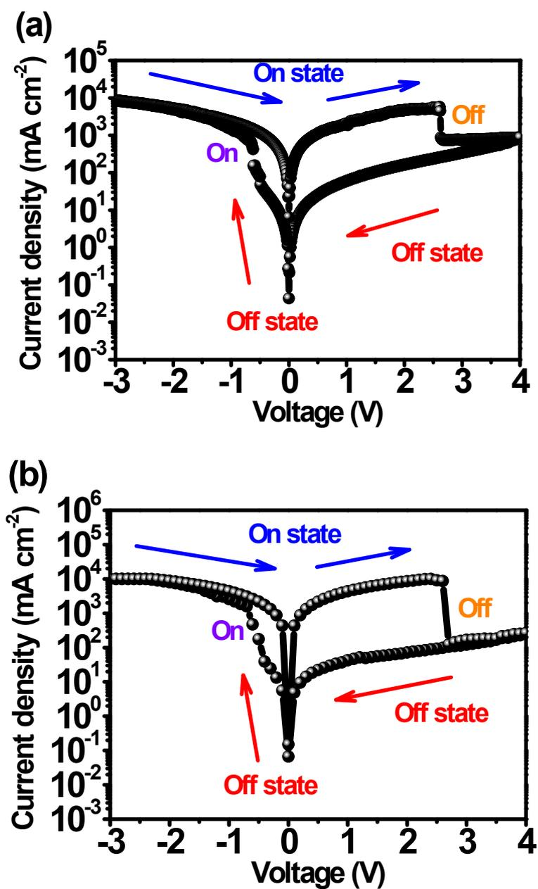
**Fig. S6** *I-V* characteristics of the memristor devices with sandwich structure. (a) ITO/PEDOT:PSS/ $\text{CH}_3\text{NH}_3\text{PbI}_{3-x}\text{Cl}_x$ /Cu. (b) ITO/PEDOT:PSS/ $\text{CH}_3\text{NH}_3\text{Pb}_{0.5}\text{Sn}_{0.5}\text{I}_3$ /Cu.
