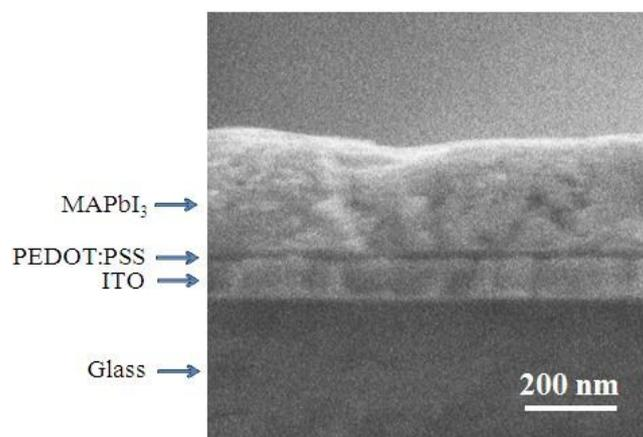
**Fig. S2** Cross-sectional SEM image of sandwiched ITO/PEDOT:PSS/CH<sub>3</sub>NH<sub>3</sub>PbI<sub>3</sub> structure without top Cu electrode.
