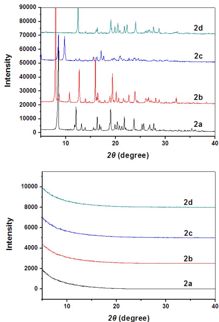
**Fig. S3** Powder XRD patterns of 2a-d in powders (upper) and Grazing incidence XRD patterns of 2a-d in films (bottom).
