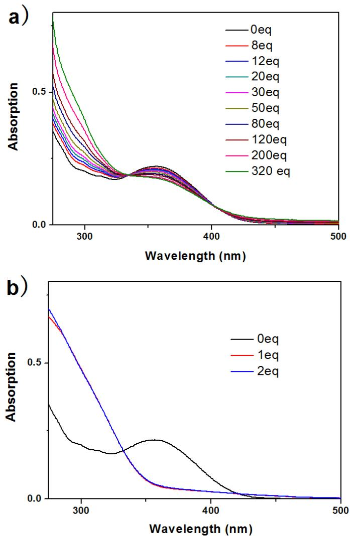
**Fig. S9** Absorption spectra of 2d (50  $\mu\text{M}$  in ACN) upon the addition of TEA (a) and TBAOH (b).
