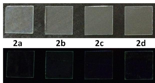
**Fig. S2** Photos of 2 in thin films prepared by spin-coating of dichloromethane solution (4 mg/ml) under natural light (upper) and UV light (bottom).
