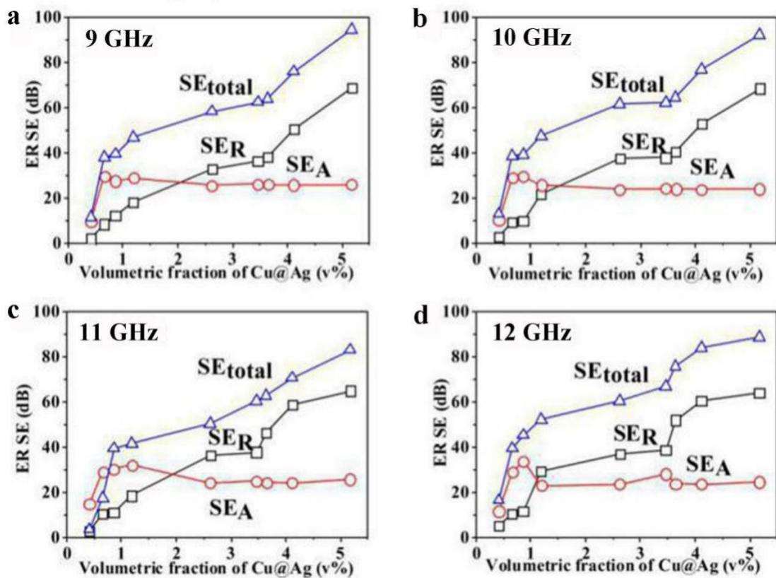
**Fig. S8.** SE<sub>total</sub>, SE<sub>A</sub> and SE<sub>R</sub> of shielding leathers in the frequencies of 9, 10, 11, and 12 GHz respectively.
