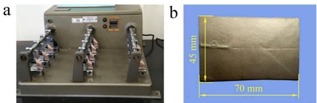
**Fig. S10.** The photos of (a) 2226 Bally Flexometer and (b) the LM-Cu@Ag (Cu@Ag 5.17 v%) after bending 25,000 times.
