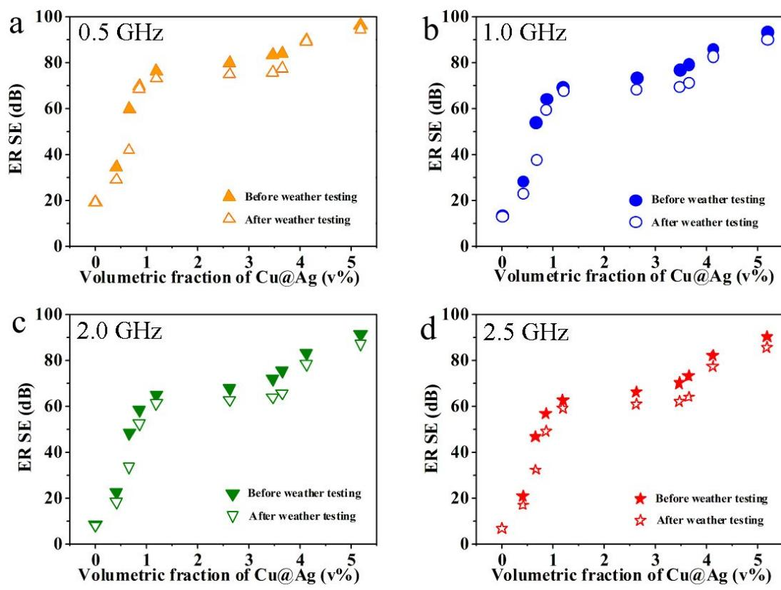
**Fig. S11.** Shielding effectiveness of LM-Cu@Ag at the typical communication frequency (0.5, 1.0, 2.0 and 2.5 GHz) before and after the weather testing.
