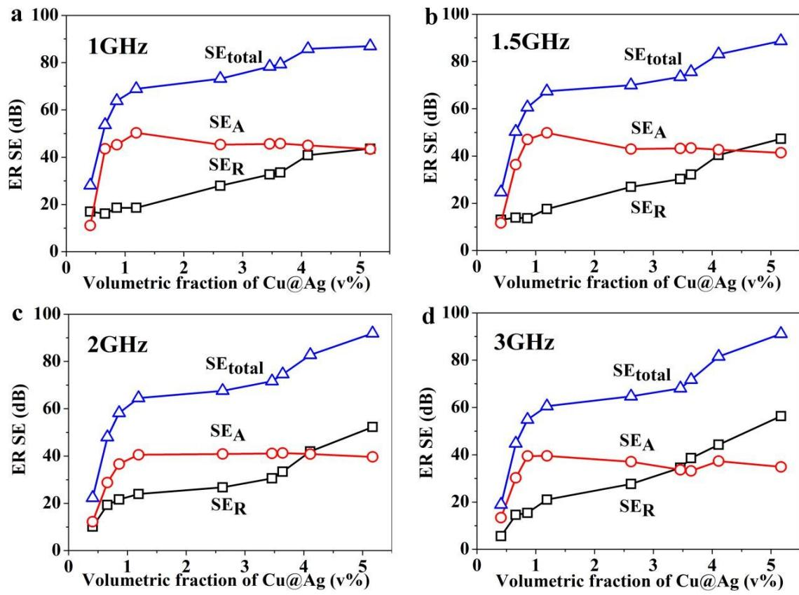
**Fig. S7.** SE<sub>total</sub>, SE<sub>A</sub> and SE<sub>R</sub> of shielding leathers in the frequencies of 1.0, 1.5, 2.0, and 3.0 GHz respectively.
