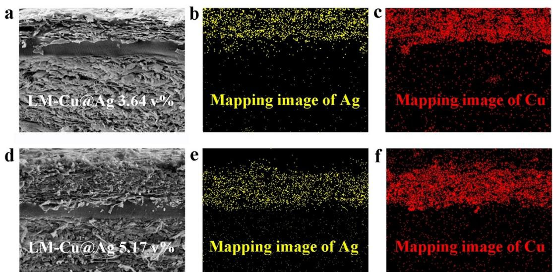
**Fig. S2.** SEM-EDX of LM-Cu@Ag with different volumetric fractions of 3.46 v% (a-c) and 5.17 v% (d-f), respectively.
