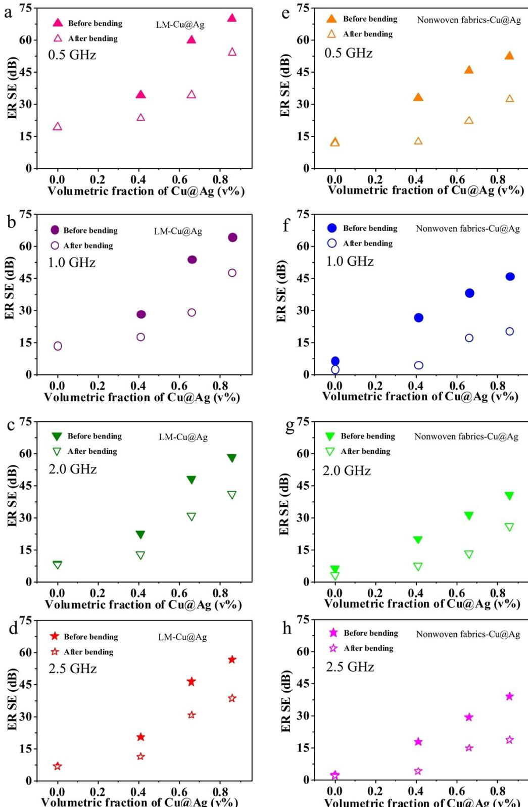
**Fig. S9.** The shielding performances of LM-Cu@Ag after bending 25,000 times. Shielding effectiveness of LM-Cu@Ag at the typical communication frequency (0.5, 1.0, 2.0 and 2.5 GHz) after bending 25,000 times (a-d). Shielding effectiveness of nonwoven fabrics-Cu@Ag at the typical communication frequency (0.5, 1.0, 2.0 and 2.5 GHz) after bending 25,000 times (e-h).
