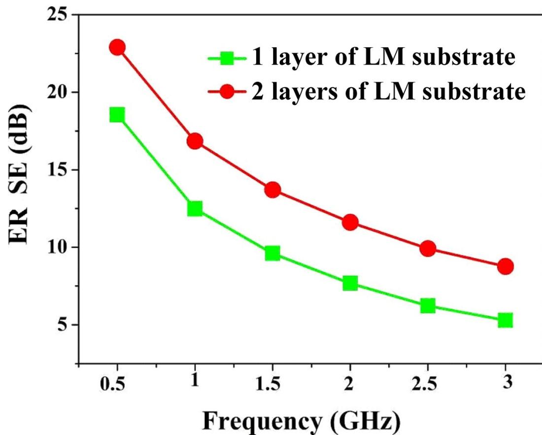
**Fig. S6.** The shielding effectiveness of LM substrate with different thickness (1 layer of LM = 0.6 mm, 2 layers of LM = 1.2 mm).
