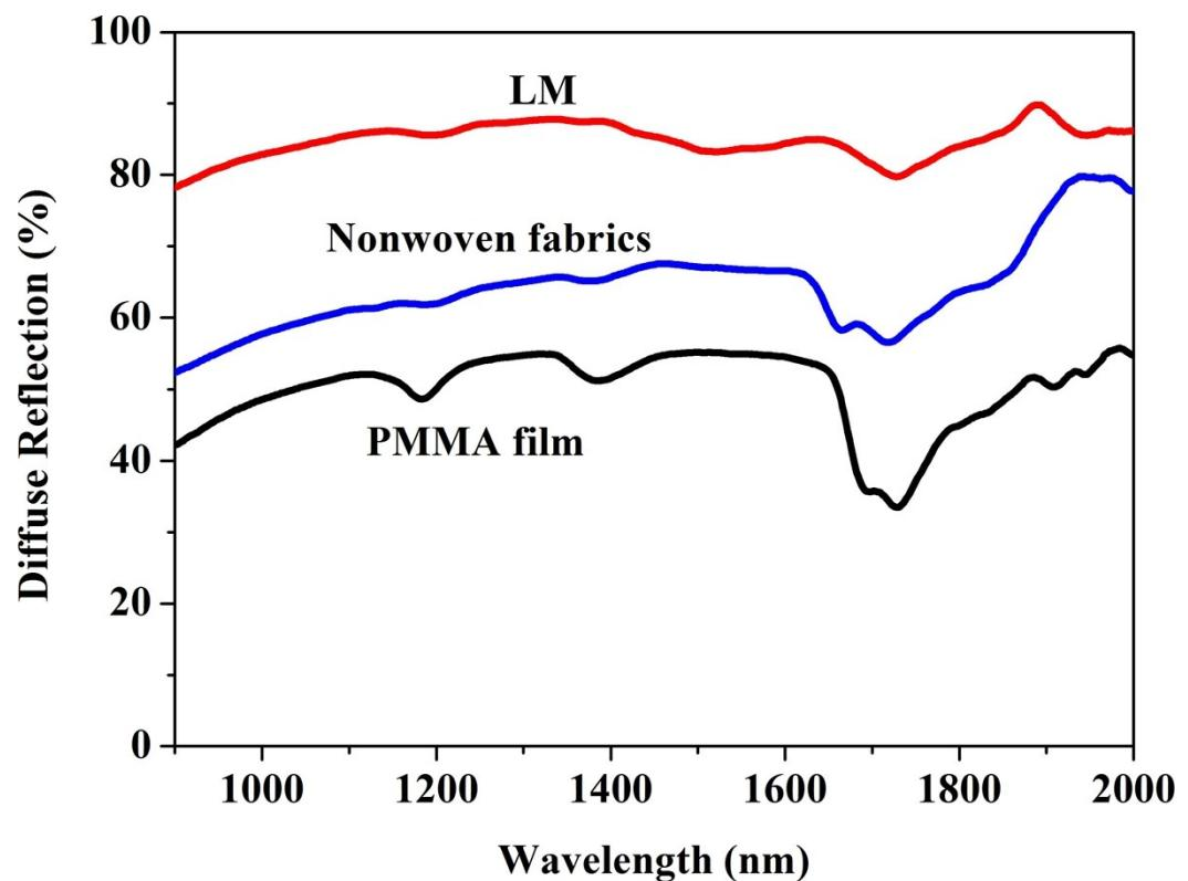
**Fig. S5.** NIR DR spectroscopy of LM, nonwoven fabrics and PMMA.
