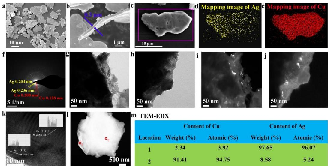
**Fig. S1.** Characterization of Cu@Ag nanoflakes. SEM images (a, b), SEM-EDX mapping images (c-e) of Cu@Ag nanoflakes, SAED pattern (f) of Cu@Ag nanoflakes, TEM image (g, h) and corresponding HADDF images (i, j) of Cu@Ag nanoflakes, HRTEM image (k) of Cu@Ag nanoflakes, TEM-EDX analyses (l, m) of Cu@Ag nanoflakes.
