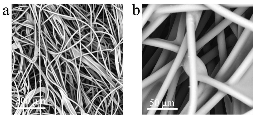
**Fig. S3.** SEM images of nonwoven fabrics at different magnifications.
