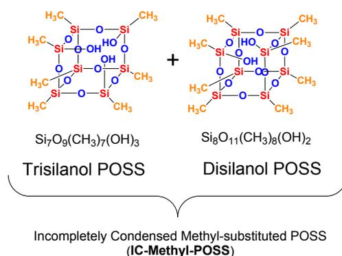
Supporting Figure S3. Chemical Structures of possible IC-Methyl POSS compounds
