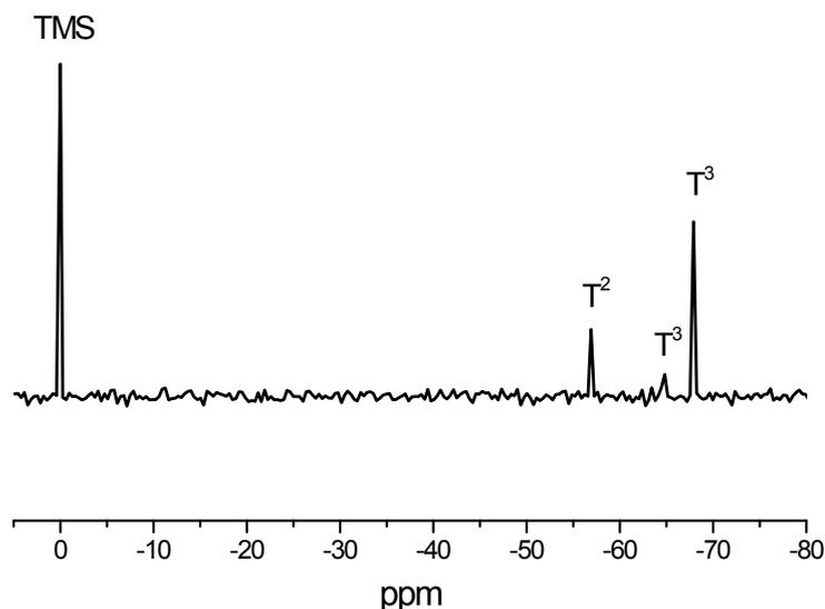
Supporting Figure S2.  $^{29}\text{Si}$  NMR spectra for IC-Methyl-POSS
