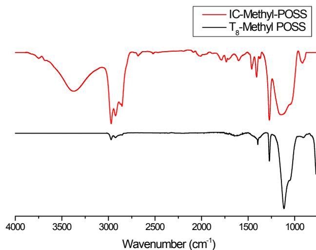
Supporting Figure S1. FTIR spectra for T<sub>8</sub>-Methyl POSS and IC-Methyl POSS
