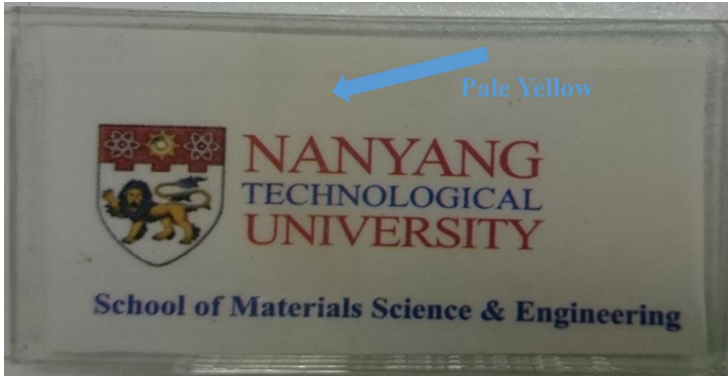
Fig. S1 Digital photo of the spray coated W_{0.71}Mo_{0.29}O_3 film showing pale-yellow color, which suggests the elimination of oxygen vacancies
