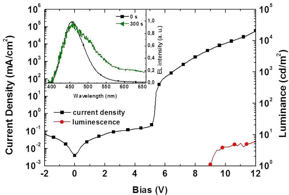
**Figure S39.** Current density (square) and luminance (circle) as a function of the bias voltage of ITO/PEDOT:PSS/7/Ca/Al devices (a) and the time-dependent evolution of the EL emission profile over the course of 5 min of continuous operation of **7** at an applied current density of  $3 \times 10^4$  mA cm<sup>-2</sup> respectively.
