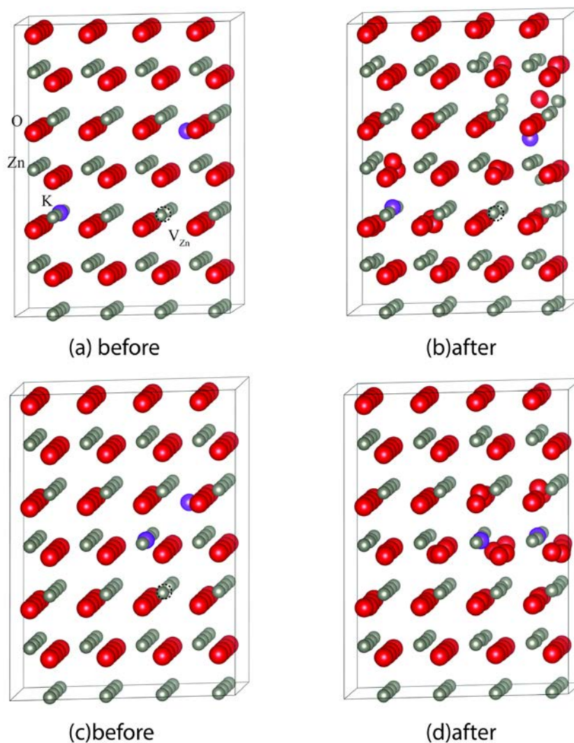
Fig. S4. Structural relaxations of ZnO supercell model with (K_{sub}+K_{int}+V_{Zn}) complex with long K-K distance 9.23 Å (a and b) and short K-K distance 6.86 Å (c and d).
