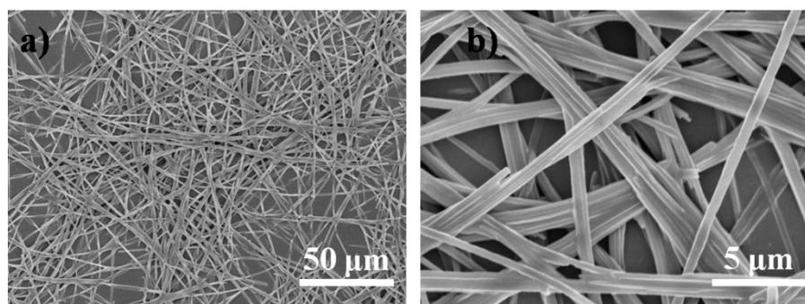
Fig. S3. SEM image of  $\text{CuPcOC}_8$  nanowires at different magnification.
