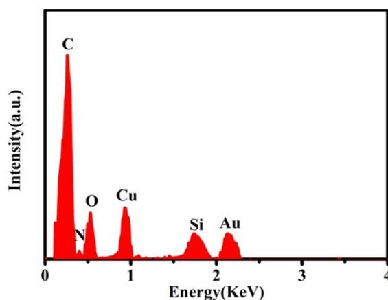
**Fig. S1.** EDX spectrum of CuPcOC<sub>4</sub> nanobelts.
