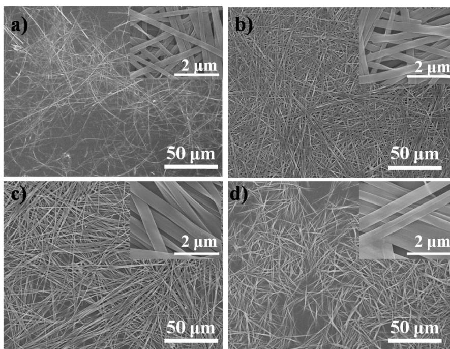
Fig. S2. SEM image of  $\text{CuPcOC}_4$  nanobelts prepared with different volume ratios of chloroform and methanol: (a) 1:5; (b) 1:10; (c) 1:20; (d) 1:40. The insets are the SEM images of corresponding samples at higher magnification.
