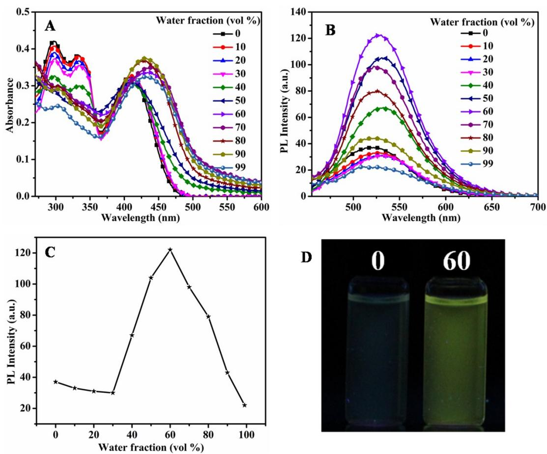
Fig. S5 The UV-vis absorption (A) and fluorescence spectra of compound **3c** in ethanol-water mixtures with different water volume fractions; the effect of water volume fraction on the maximum emission intensity (C); optical photographs recorded under 365 nm UV irradiation with various fractions of water (D).
