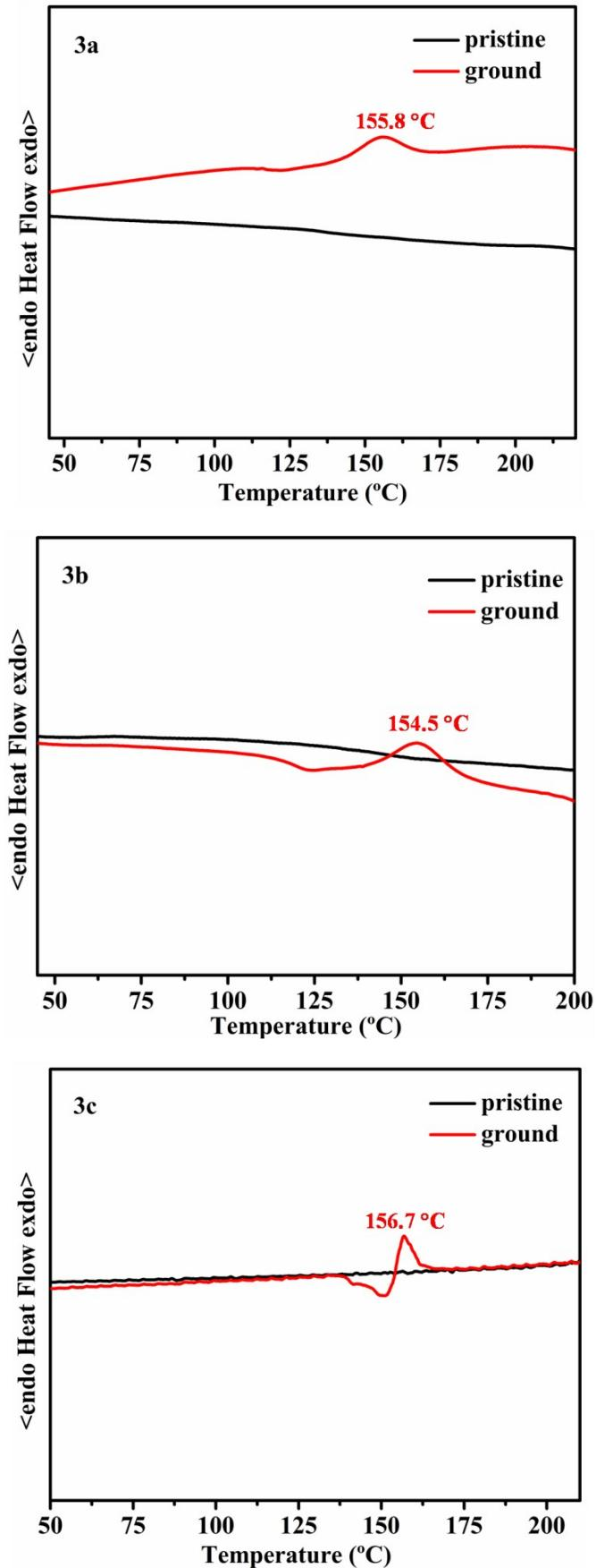
Fig. S10 DSC curves of **3a**-**3c** in the pristine and ground powders. (scan rate: 10 °C min<sup>-1</sup>)
