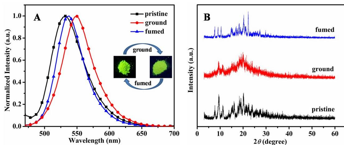
Fig. S8 Emission spectra (A) and XRD patterns (B) of pristine, ground and fumed with ethanol of compound **3b**. Inset: photographs of pristine and ground powders under 365 nm light.
