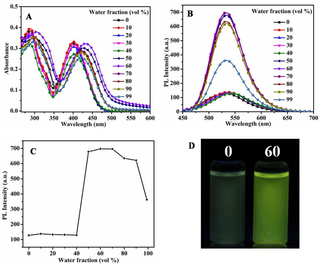
Fig. S4 The UV-vis absorption (A) and fluorescence spectra of compound **3b** in ethanol-water mixtures with different water volume fractions; the effect of water volume fraction on the maximum emission intensity (C); optical photographs recorded under 365 nm UV irradiation with various fractions of water (D).
