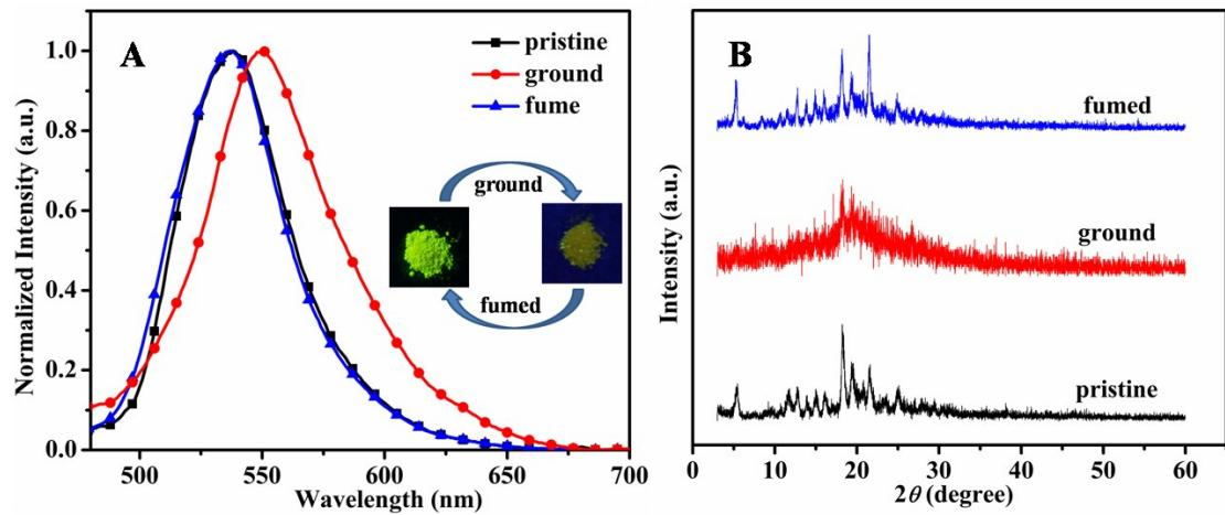
Fig. S9 Emission spectra (A) and XRD patterns (B) of pristine, ground and fumed with ethanol of compound **3c**. Inset: photographs of pristine and ground powders under 365 nm light.
