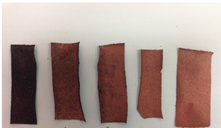
Fig. S1 From left to right, color of each cotton fabric sample at different ELD plating time 30 , 60, 90, 120 and 150 min
