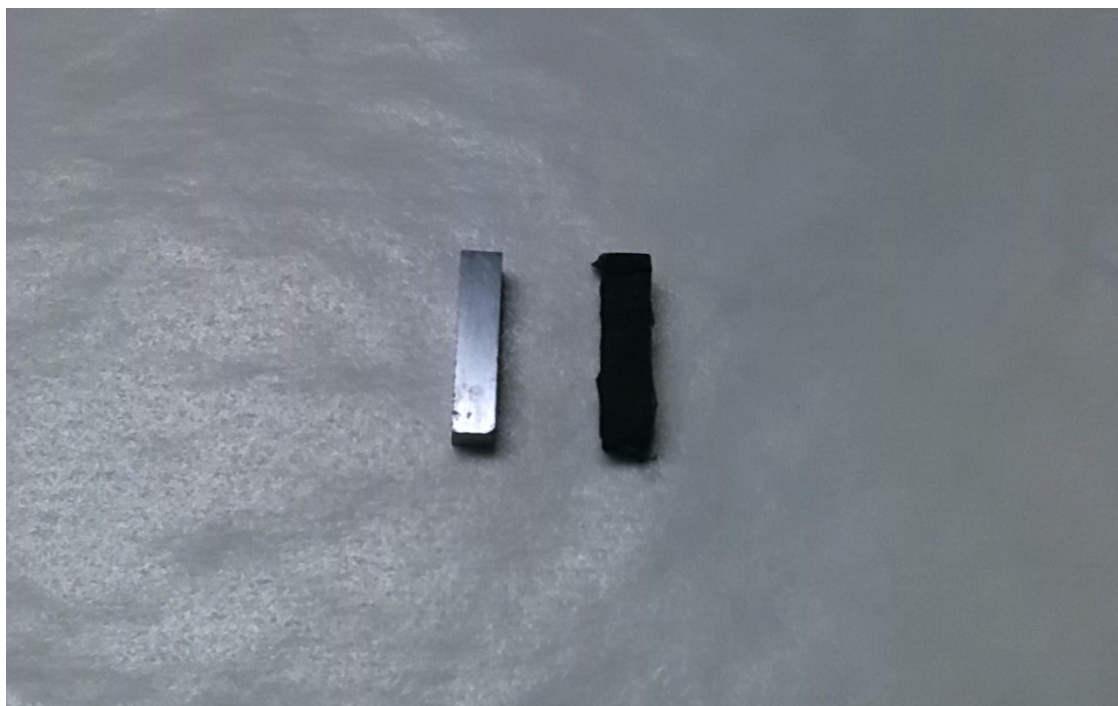
Fig. S5 Photo of two pieces of sample from the same pellet (the one the left is the one that has not been tested and the one on the right is the one that has been measured to 775K.)
