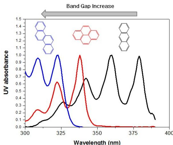
Fig S1. UV-vis absorption normalized spectra of anthracene, pyrene and chrysene in solution state.
