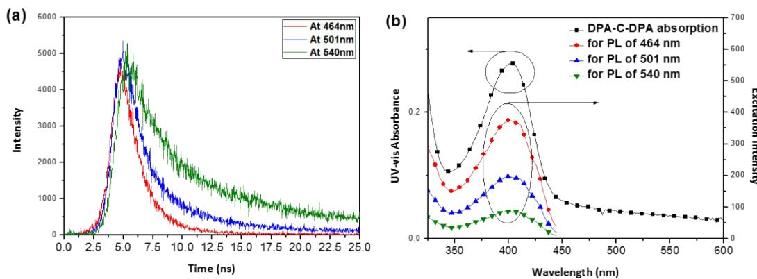
**Fig S7.** (a) Time-resolved emission decays, (b) UV-vis absorption spectrum and excitation spectra of DPA-C-DPA film (thickness: 100nm).
