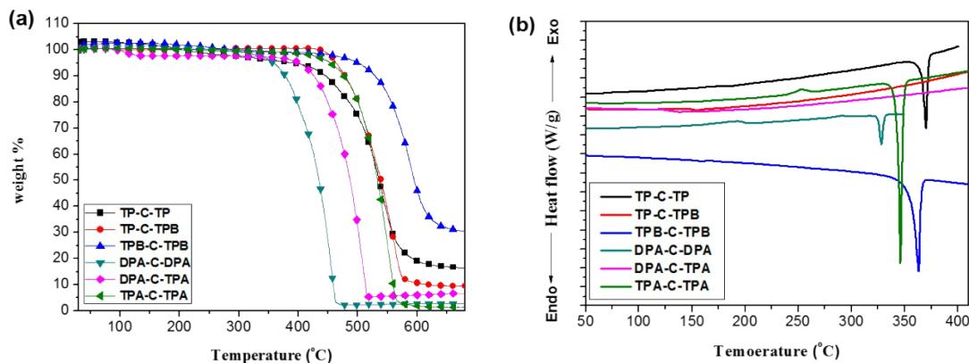
**Fig S4.** Thermal properties of chrysene derivatives. (a) TGA curves, (b) DSC curves.
