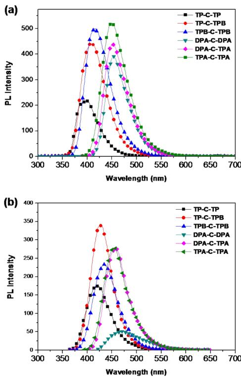
**Fig S6.** PL spectra of chrysene derivatives: (a) solution state, (b) film state.
