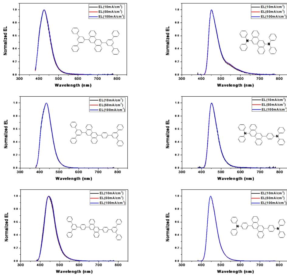
**Fig S8.** Normalized EL spectra of synthesized compounds.**Table S1.** Optical properties of anthracene, pyrene and chrysene core compounds.
