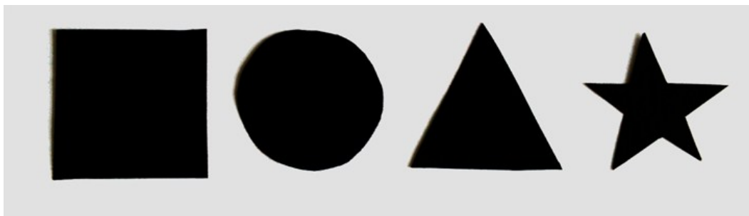
Fig. S1 The PPy/SWCNT composite films can be easily cut into a variety of shapes including squares, circles, triangles and stars.
