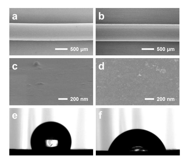
Figure S3. (a) SEM image of black spandex fiber. (b) SEM image of oxygen plasmatreated black spandex fiber. (c) SEM image of (a) at a higher magnification. (d) SEM image of (b) at a higher magnification. (e) and (f) The water contact angle of spandex fiber before (e) and after (f) oxygen plasma treatment.
