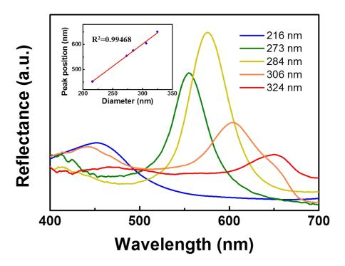
**Figure S8.** Reflection spectra of the MCFs containing PS/PMMA/PEA core-shell microspheres with different diameters (inset, experimental correlation between the peak position and microsphere diameter).
