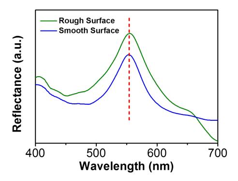
**Figure S9.** Reflection spectra of MCFs from multi-ply fibers with the rough surface and single-ply fiber with smooth surface.
