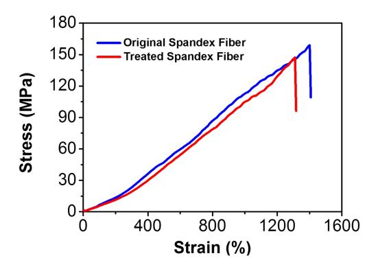
**Figure S4.** Stress-strain curves of the spandex fibers before and after oxygen plasma treatment.
