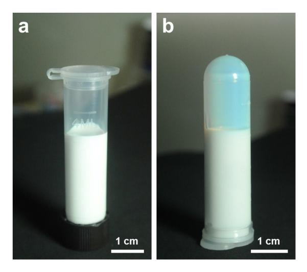
**Figure S2.** Photographs of the concentrated PS/PMMA/PEA core-shell microsphere dispersion that had been stored for 4 months.
