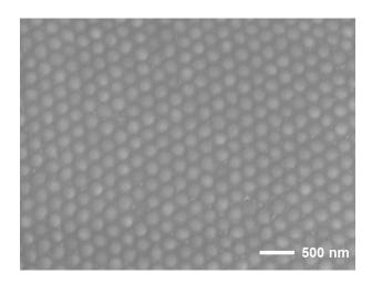
**Figure S6.** SEM image of PS/PMMA/PEA core-shell microspheres on a planar glass substrate.
