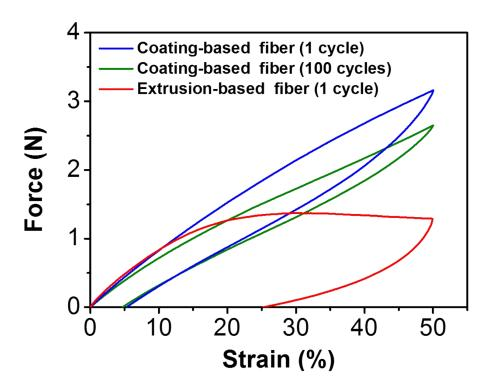
**Figure S13.** Stress-strain curves in the stretching and releasing cycles for coatingbased and extrusion-based MCFs with a strain of 50%.
