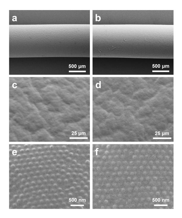
Figure S14. (a) and (b) SEM images of a MCFs before and after a standard laundry process in the washing machine. (c) and (e) Higher magnification of (a). (d) and (f) Higher magnification of (b).
