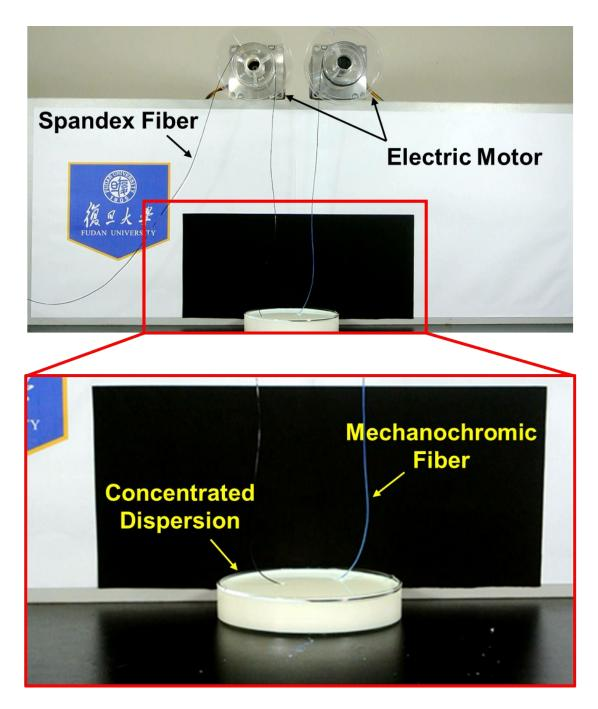
Figure S1. Photograph of the continuous preparation of MCFs.
