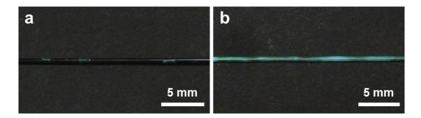
**Figure S7.** (a) Photograph of a MCF based on the microsphere dispersion with a lower solid content of ~31 %. (b) Photograph of a MCF based on the spandex fiber without plasma treatment.
