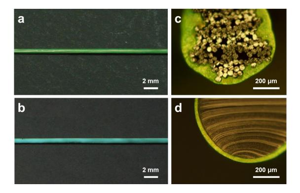
**Figure S10**. (**a**) and (**b**) Photographs of MCFs based on the multi-ply and single-ply fiber, respectively. (**c**) and (**d**) Cross-sectional optical micrographs of MCFs based on the multi-ply fiber at (**a**) and single-ply fiber at (**b**), respectively.
