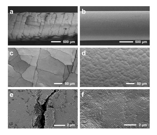
**Figure S5.** (**a**) and (**b**) SEM images of MCFs from PS microspheres with a diameter of 240 nm and PS/PMMA/PEA core-shell microspheres, respectively. (**c**) and (**e**) Higher magnification of (**a**). (**d**) and (**f**) Higher magnification of (**b**).
