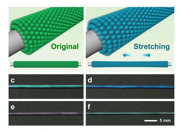
Figure S11. (a) and (b) Schematic illustrations to the mechanochromic behavior of the composite fiber before and after stretching, respectively. (c) and (d) Photographs of the fiber with colors of green and blue before and after stretching, respectively. (e) and (f) Photographs of the fiber with colors of red and green before and after stretching, respectively.
