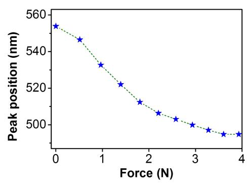
Figure S12. The variation of reflection peak position of MCFs with increasing forces.
