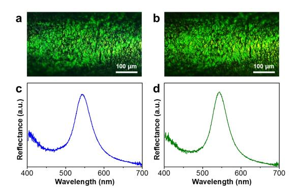
Figure S15. (a) and (b) Optical micrographs of MCF before and after a standard wash machine process, respectively. (c) and (d) Reflection spectra of fiber at (a) and (b), respectively.
