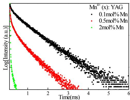
**Figure S6.** Mn<sup>4+</sup> content dependent decay curves of Mn<sup>4+</sup>: <sup>2</sup>E state ( $\lambda_{em}$ = 673 nm) in Mn<sup>4+</sup>: YAG under 352 nm light excitation.
