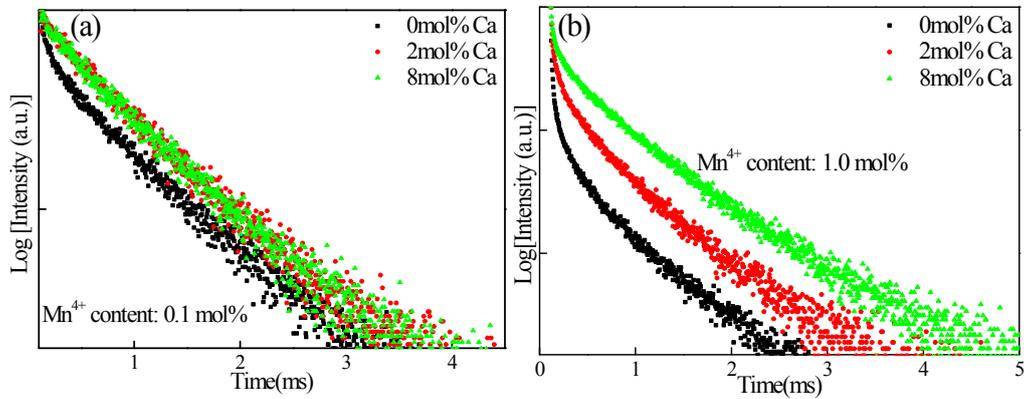
**Figure S4.** Decay curves of  $\text{Mn}^{4+}$ :  ${}^2\text{E}$  excited state ( $\lambda_{\text{em}}=673$  nm) in (a)  $\text{Mn}^{4+}/\text{Ca}^{2+}$ (0.1/y, mol%): YAG and (b)  $\text{Mn}^{4+}/\text{Ca}^{2+}$  (1.0/y, mol%): YAG (y=0, 2, 8) under 352 nm UV light excitation.
