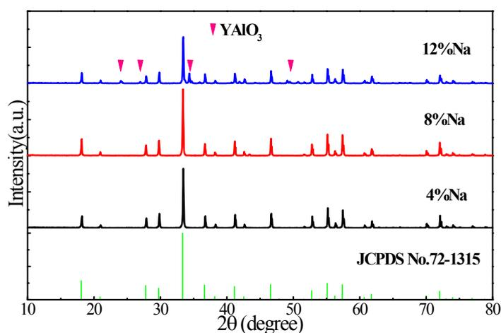
**Figure S1.** XRD patterns of Mn<sup>4+</sup>/Na<sup>+</sup> (0.1/y, mol%): YAG (y= 4, 8, 12) phosphors
