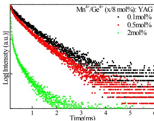
**Figure S8.** Mn<sup>4+</sup> content dependent decay curves of Mn<sup>4+</sup>: <sup>2</sup>E state ( $\lambda_{em}$ = 673 nm) in Mn<sup>4+</sup>/Ge<sup>4+</sup>: YAG under 352 nm light excitation.
