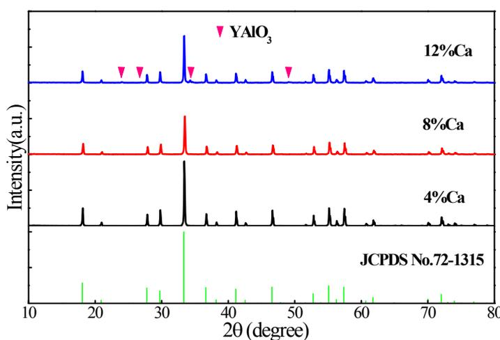
**Figure S2.** XRD patterns of Mn<sup>4+</sup>/Ca<sup>2+</sup> (0.1/y, mol%): YAG (y= 4, 8, 12) phosphors
