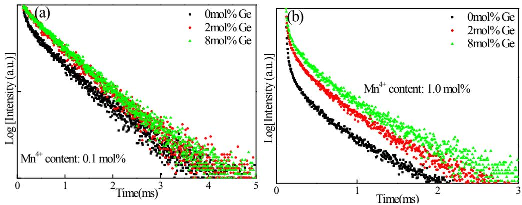
**Figure S5.** Decay curves of  $\text{Mn}^{4+}$ :  ${}^2\text{E}$  excited state ( $\lambda_{\text{em}}=673$  nm) in (a)  $\text{Mn}^{4+}/\text{Ge}^{4+}$ (0.1/y, mol%): YAG and (b)  $\text{Mn}^{4+}/\text{Ge}^{4+}$  (1.0/y, mol%): YAG (y=0, 2, 8) under 352 nm UV light excitation.
