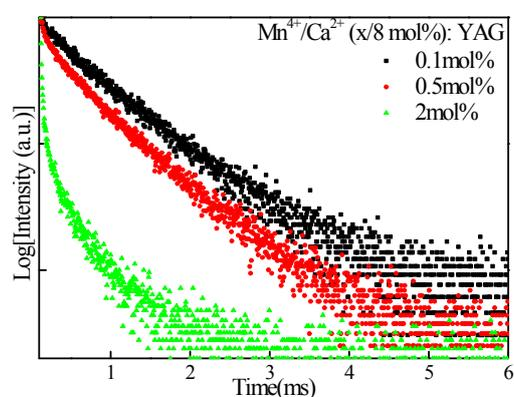
**Figure S7.** Mn<sup>4+</sup> content dependent decay curves of Mn<sup>4+</sup>: <sup>2</sup>E state ( $\lambda_{em}$ = 673 nm) in Mn<sup>4+</sup>/Ca<sup>2+</sup>: YAG under 352 nm light excitation.
