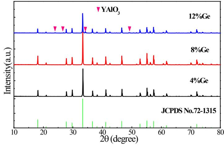
**Figure S3.** XRD patterns of  $\text{Mn}^{4+}/\text{Ge}^{4+}$  (0.1/y, mol%): YAG (y= 4, 8, 12) phosphors
