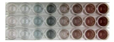
Figure S1 Photographs of the AuNRs growth solution after the addition of different amount of ALP-antibody conjugates. The original solution of ALP-antibody conjugates in the ELISA kit was diluted for 2500 times with 1 mM Tris-HCl buffer (pH7.4) . The amounts of diluted ALP-antibody conjugates added from left to right were 0, 10, 20, 30, 40, 50, 60, 70  $\mu$ L, respectively, and three replicates were conducted for each sample.
