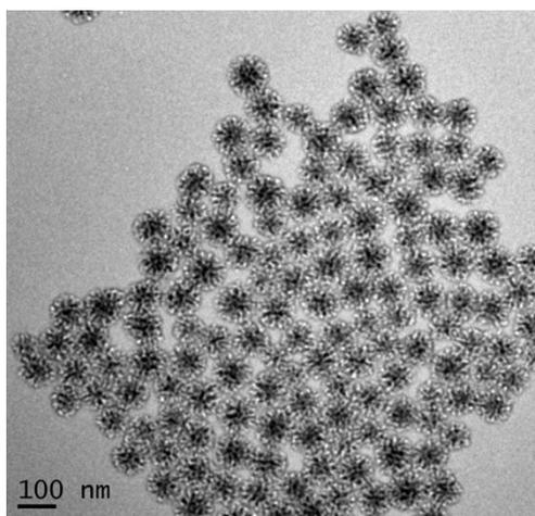
**Fig. S1** TEM image of PCMSNs synthesized (about 80 nm)
