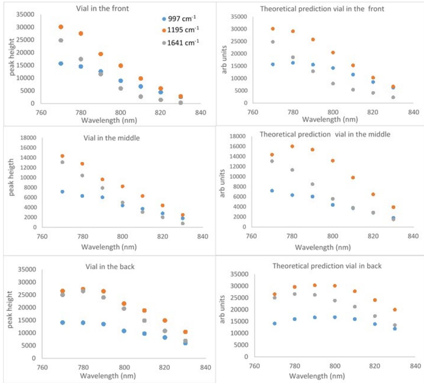
Figure S5 Experimental Raman peak height vs laser wavelength for each position of the vial [left hand side] inside the tissue along their theoretical predictions of Raman peak height (right hand side)
