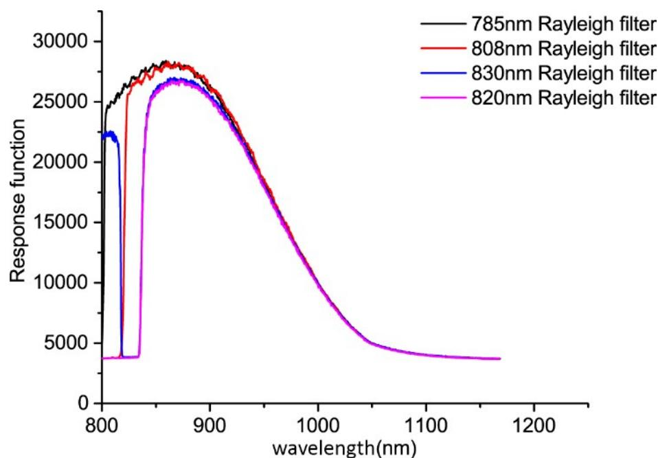
Figure S1 instruments response function including the intermediary optics used. Each one of the plot corresponds to a long pass filter used to reject laser scattering at different wavelengths.
