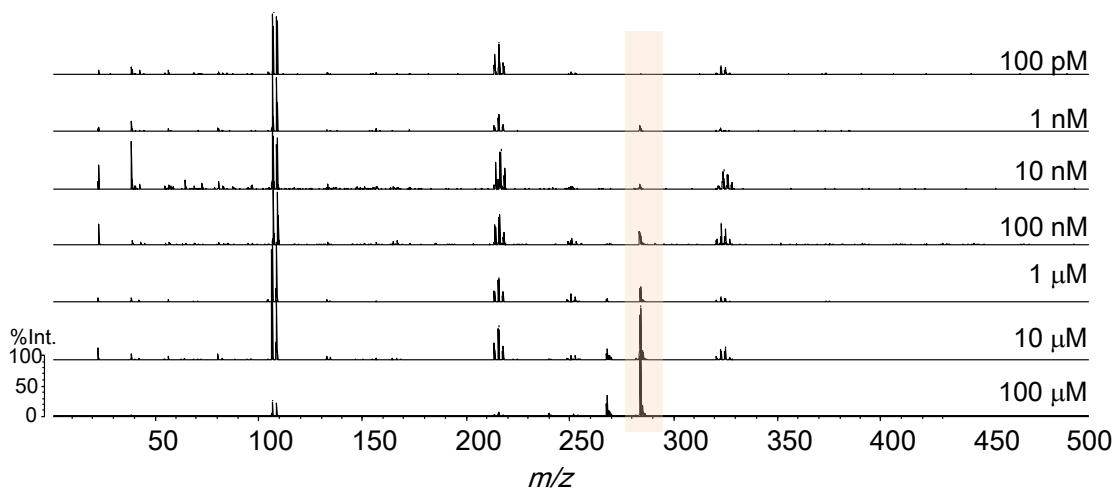
**Figure S5** SALDI mass spectra of MB on the Ag NP-GF substrate with  $35 \mu\text{g}/\text{cm}^2$  obtained from different concentrations of MB.
