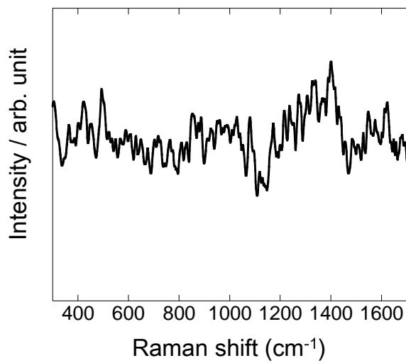
**Figure S3.** SERS spectrum of 4-ATP (1  $\mu\text{M}$ ) on the AgNP-functionalized glass “plate” with 35  $\mu\text{g}/\text{cm}^2$  Ag.
