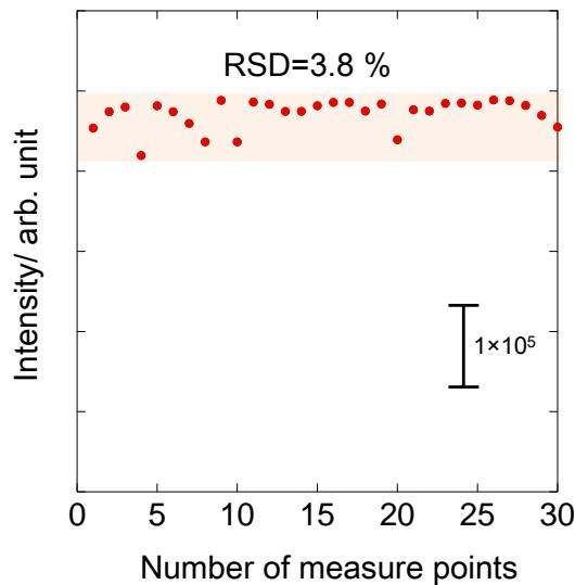
**Figure S1** SERS peak intensities of 4-ATP at  $1064\text{ cm}^{-1}$  on the Ag NP-GF substrates with  $35\text{ }\mu\text{g}/\text{cm}^2$  of Ag. The standard error obtained from 30 different locations is 3.8 % in the Raman signals. Before the SERS measurements, the Ag NP-GF substrates were immersed in  $100\text{ }\mu\text{M}$  4-ATP solution.
