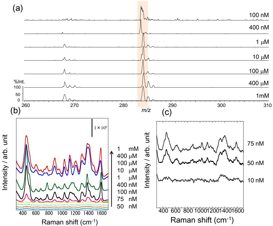
**Figure S4.** (a) SALDI mass spectra of MB on the Ag NP-GF substrate with 35  $\mu\text{g}/\text{cm}^2$  obtained from different concentrations of MB. (b), (c) SERS spectra of MB on the the Ag NP-GF substrate with 35  $\mu\text{g}/\text{cm}^2$  obtained from different concentrations of MB. Herein, the SALDI signal intensities of MB at  $m/z = 284$  [ $\text{M}-\text{Cl}]^+$  and the Raman intensities of MB at 451  $\text{cm}^{-1}$  were used in the evaluation of enhanced factors.
