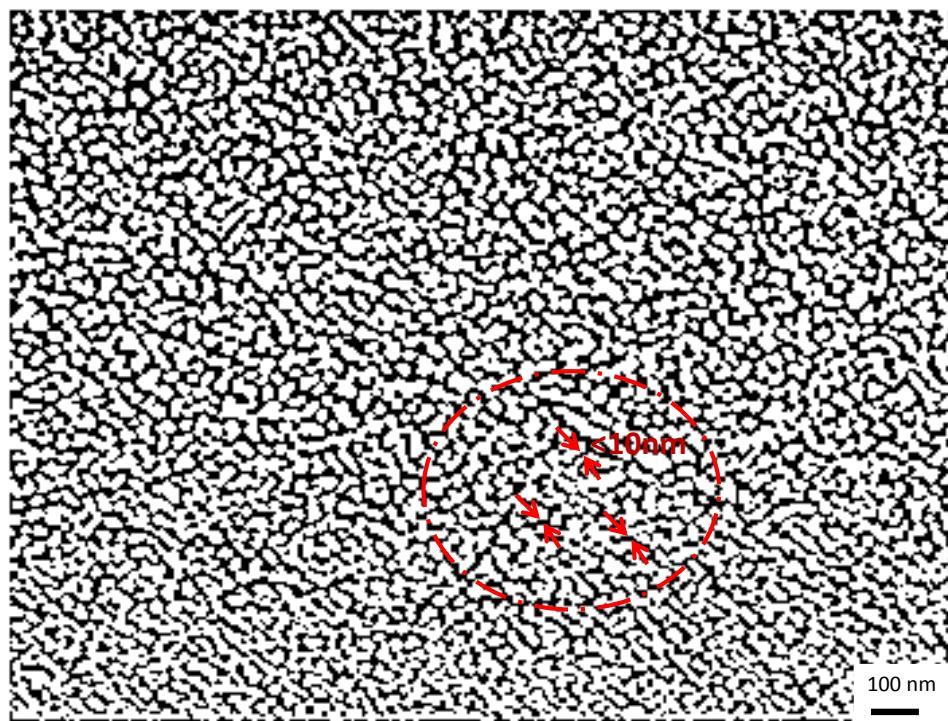
**Figure S2** Binary image of the SEM image (Fig. 2b in the main text). We measured the inter-particle distance from the binary image and confirmed the presence of many inter-particle nanoscale gaps  $< 10\text{ nm}$  in the substrate as shown in red arrows in the figure.
