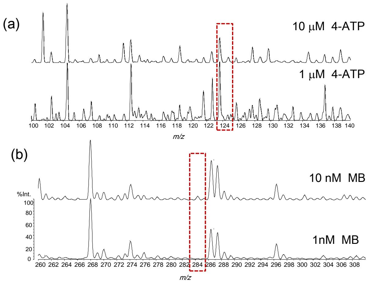
**Figure S7.** MALDI spectra of (a) 4-ATP and (b) MB on the bare glass fibers using CHCA matrix (10 mg/ mL). The peaks of 4-ATP ( $[M-H]^+$  at  $m/z = 124$ ) and MB ( $[M-Cl]^+$  at  $m/z 284$ ) both were not detectable at the concentrations in the MALDI-MS.
