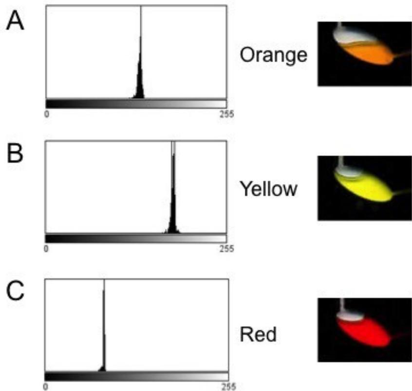
**SI Figure 1. Histograms from dye studies.** **A)** Orange dye was mixed off-chip using the same ratio of yellow: red dye (4:1) that was used in Fig. 2B and added to the LAMP chamber. **B)** Yellow dye was added to the LAMP chamber. **C)** Red dye was added to LAMP chamber.
