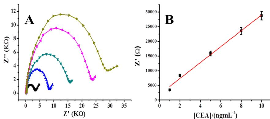
**Figure S3.** EIS of the CEA aptamer modified Au electrode incubated with different concentration of CEA from 1 to 10 ng/mL in 0.1 M NaCl+5 mM  $Fe(CN)_6^{3-/4-}$  solution.
