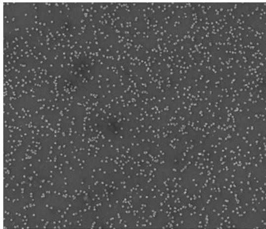
**Figure S2.** The SEM image of the ITO electrode surface electrodeposited with Au.
