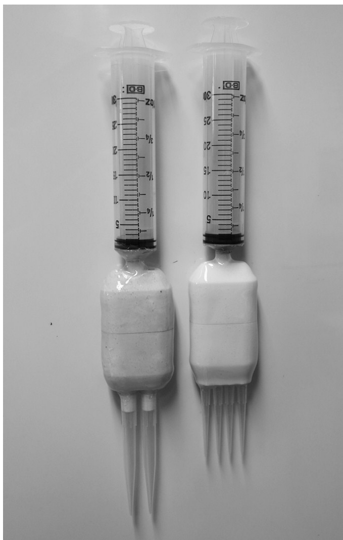
FIG. S1. A photograph of smart multi-pipettes with two and four liquid-holding nozzles. The four-nozzle smart pipette is composed of four 200- \mu L pipette tips and can deliver four different fluids into a microfluidic device. Customized nozzles with narrow ends can be further integrated to increase the number of the nozzles.
