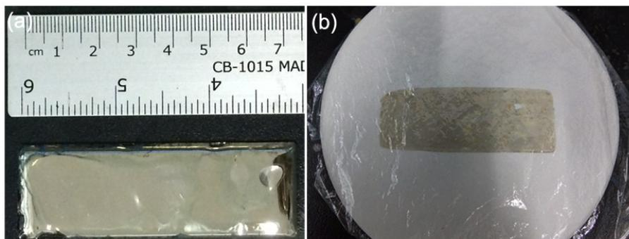
Fig. S1 Photograph of (a) the resultant Ag-NCs monolayer covered at the glass slide (b) the Ag-NCs monolayer coated on the PE film.
