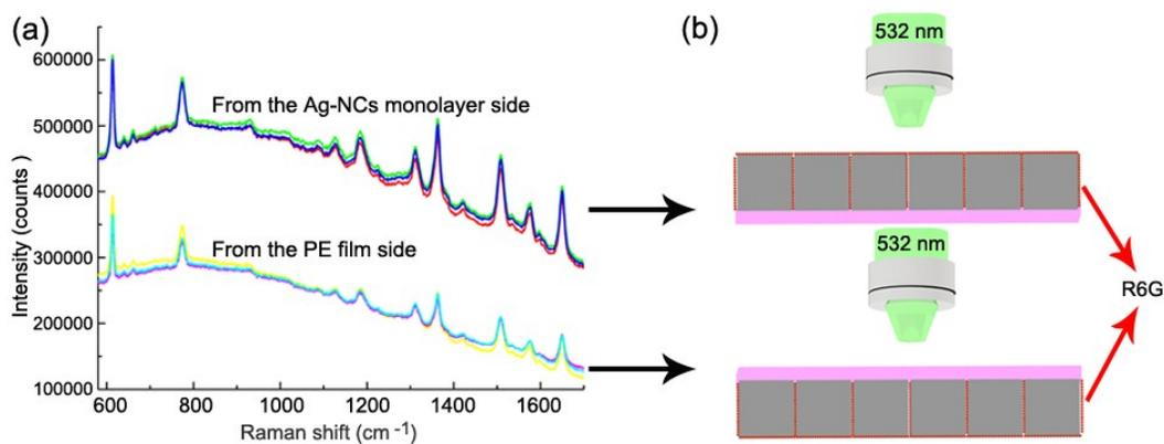
Fig. S6 (a) SERS spectra of R6G (1  $\mu\text{M}$ ) collected from both side of the Ag-NCs@PE composite film at the excitation wavelength of 532 nm. (b) Schematic detection process in Fig. S6a.
