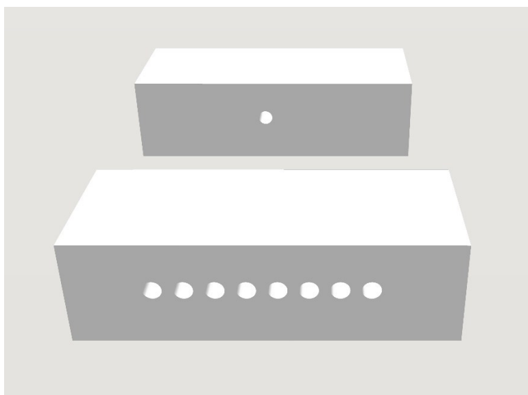
Figure S-4. 3D renderings of 8-port fluidic manifold, allowing one vacuum line to control 8 independent lines. The top rendering is a view from the vacuum port, and the bottom rendering is a view from the 8-tube port that interfaces with the 8 microfluidic channels of the device shown in Figure 1 of the main text. This manifold was also interfaced with the 8-strip sample collection device shown in Figure 1 of the main text and in Figure S-3 above. (STL and SKP files: “8 channel manifold RSC”)
