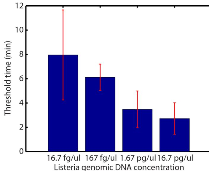
**Figure S4.** Results of the ITP-RPA assay using purified *L. Monocytogenes* genomic DNA spiked into whole blood. We here quantify threshold times as determined by the Opticon Monitor software. Error bars represent 95% confidence on the mean (from Student's t-distribution).
