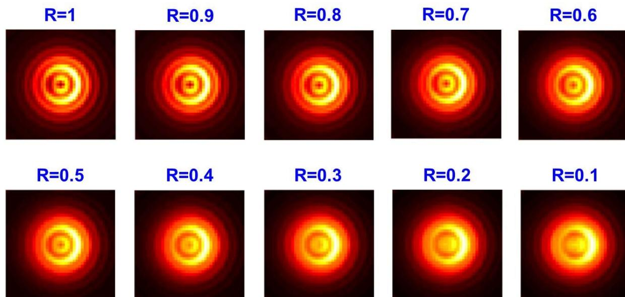
**Fig. S10** The simulated defocused scattering patterns of a AuNR by varying the parameter  $R$  from 1 to 0.1. In this simulation, the polar angle  $\theta$  of a Pt-AuNR1 was set to  $57^\circ$ . A solid bright spot at the center of the doughnut-shaped scattering pattern is clearly appeared with decreasing the  $R$  value.
