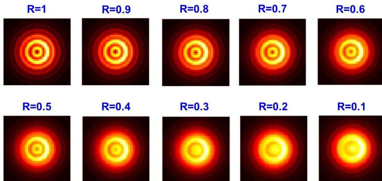
**Fig. S11** The simulated defocused scattering patterns of a AuNR by varying the parameter  $R$  from 1 to 0.1. In this simulation, the polar angle  $\theta$  of a Pd-AuNR1 was set to  $73^\circ$ . A solid bright spot at the center of the doughnut-shaped scattering pattern is clearly appeared with decreasing the  $R$  value.
