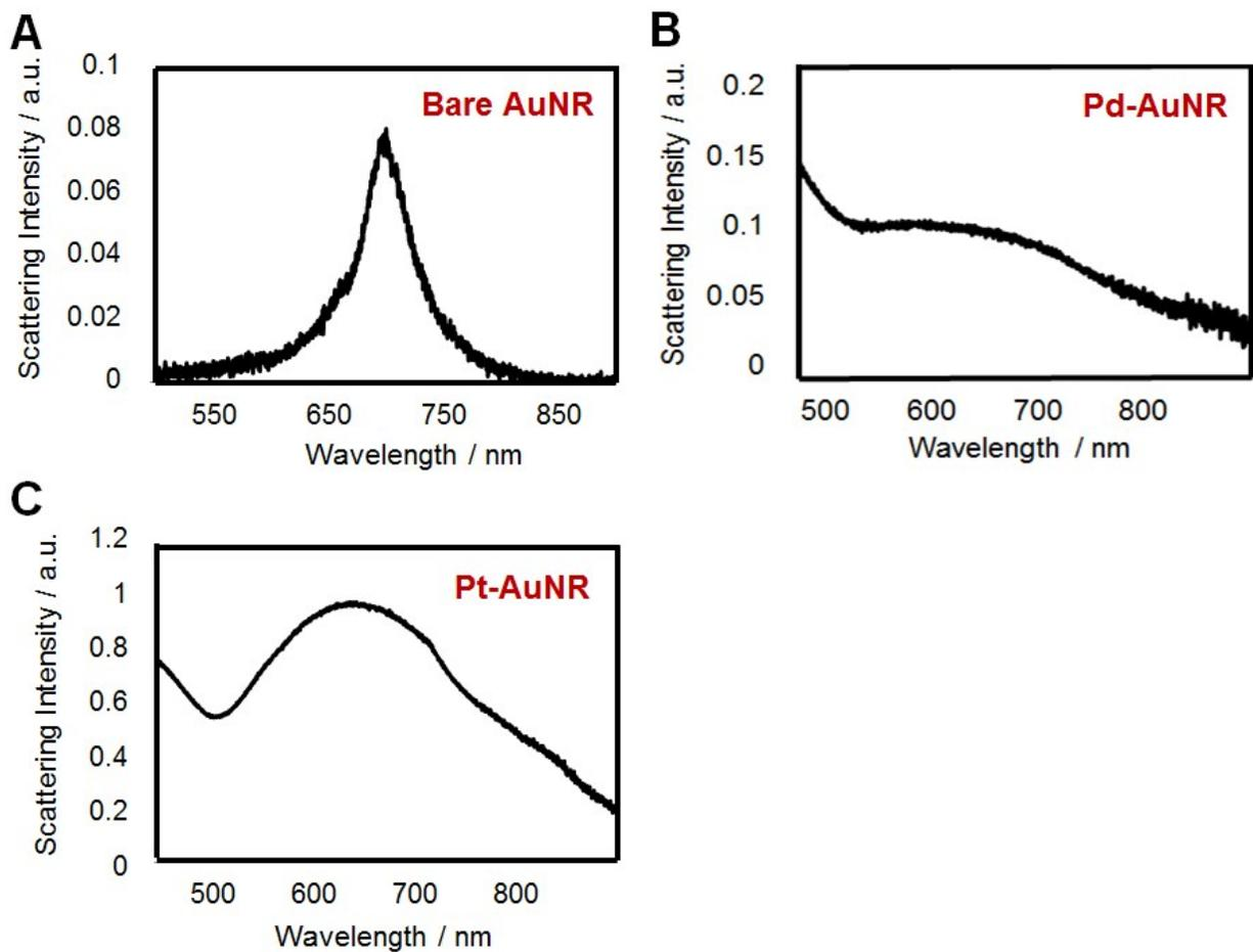
**Fig. S4** Single particle scattering spectra of (A) bare AuNR, (B) Pd-AuNR, and (C) Pt-AuNR. The strong plasmon damping is observed for the hybrid bimetallic AuNRs with the much increased LSPR linewidth.
