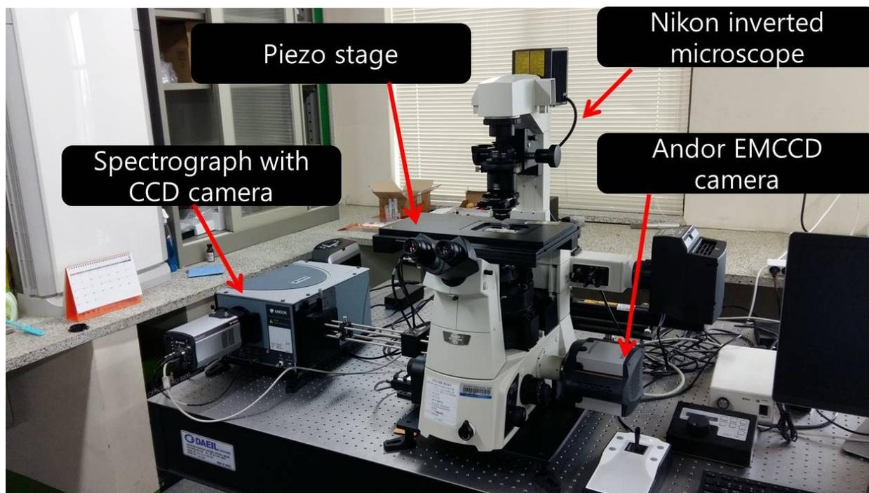
**Fig. S3** Experimental setup for single particle microscopy and spectroscopy.
