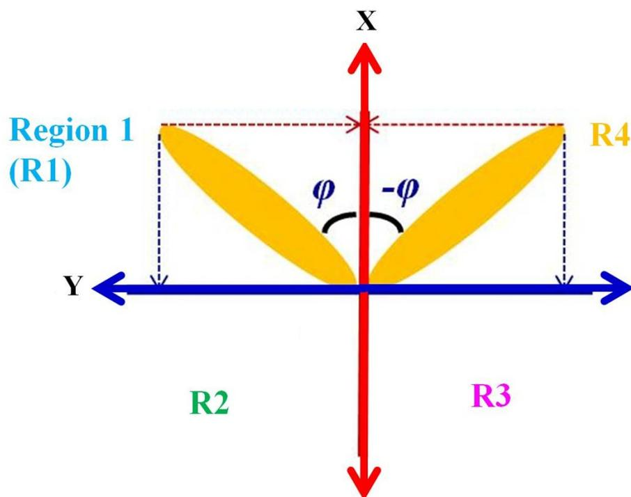
**Fig. S7** Schematic diagram to show angular degeneracy generally considered a major limitation of polarization-based techniques in single particle rotational tracking. The angular degeneracy is resulted from the 2-fold optical symmetry of a AuNR relative to the x-axis (red-arrow). We cannot distinguish the orientation angle between  $\varphi$  and  $-\varphi$  with the respect to x- axis.
