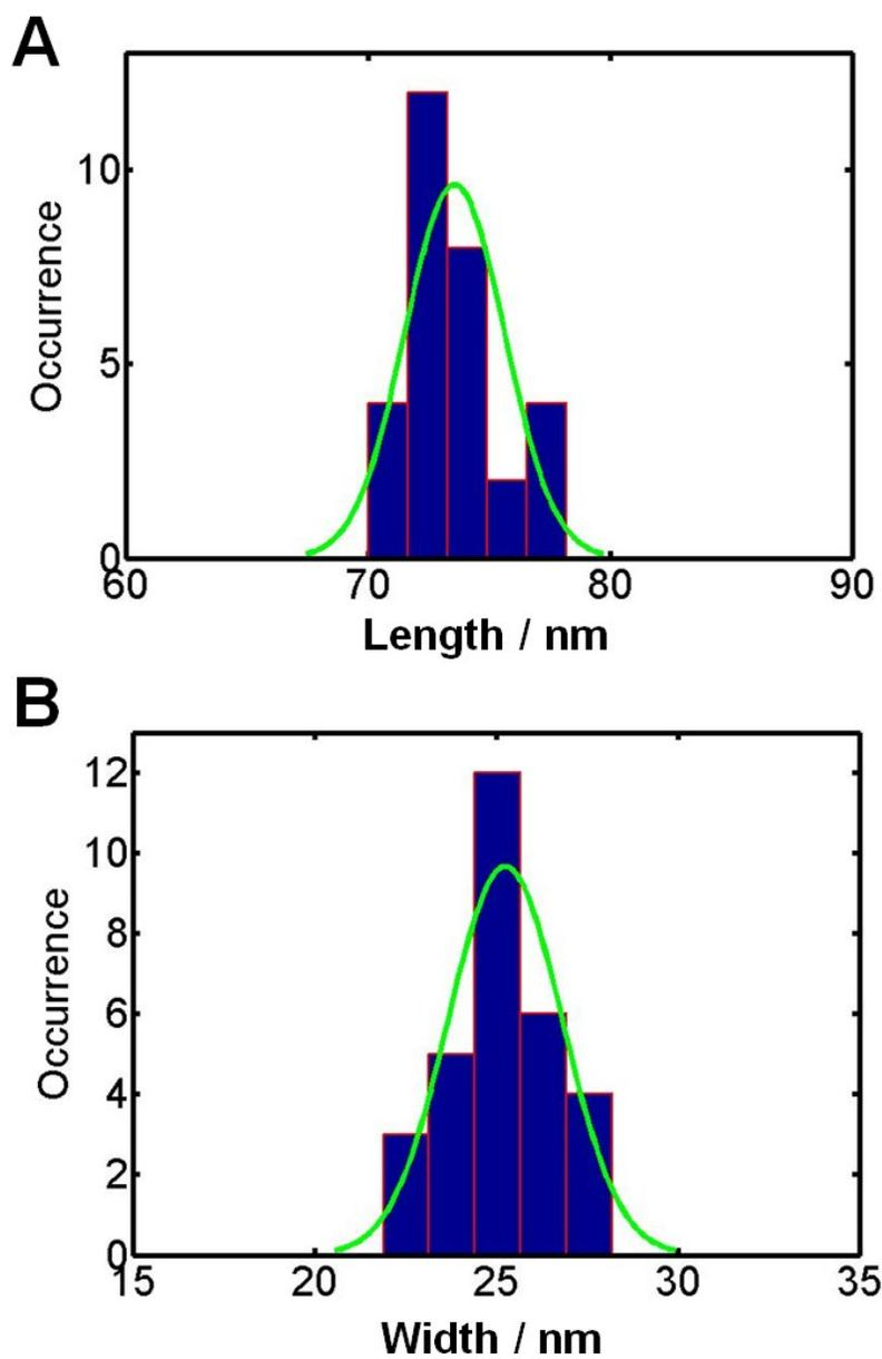
**Fig. S1** Size distribution of bimetallic AuNRs. The average length and width are  $73.6(\pm 2.14)$  nm and  $25.3(\pm 1.56)$  nm, respectively.
