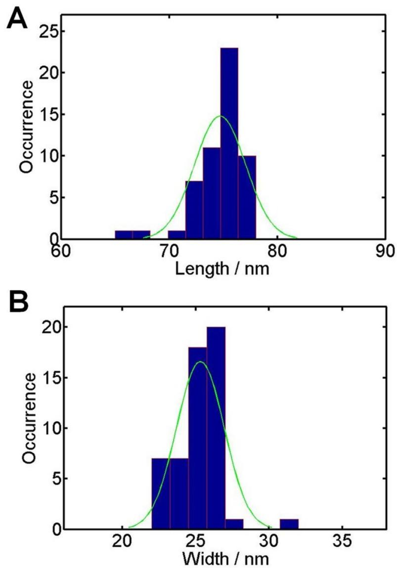
**Fig. S2** Size distribution of bare AuNRs. The average length and width are  $73.7(\pm 3.38)$  nm and  $25.4(\pm 1.65)$  nm, respectively.
