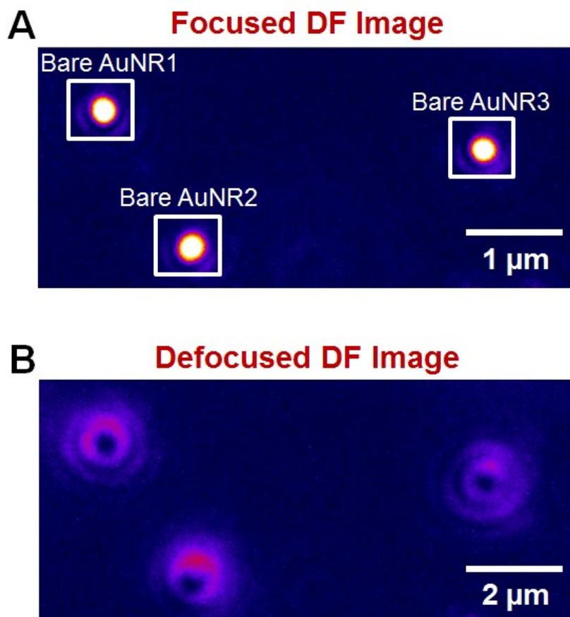
**Fig. S8** (A) Focused DF image of bare AuNRs. (B) Defocused DF image for the same AuNRs at the defocusing distance of  $\sim 1 \mu\text{m}$ .
