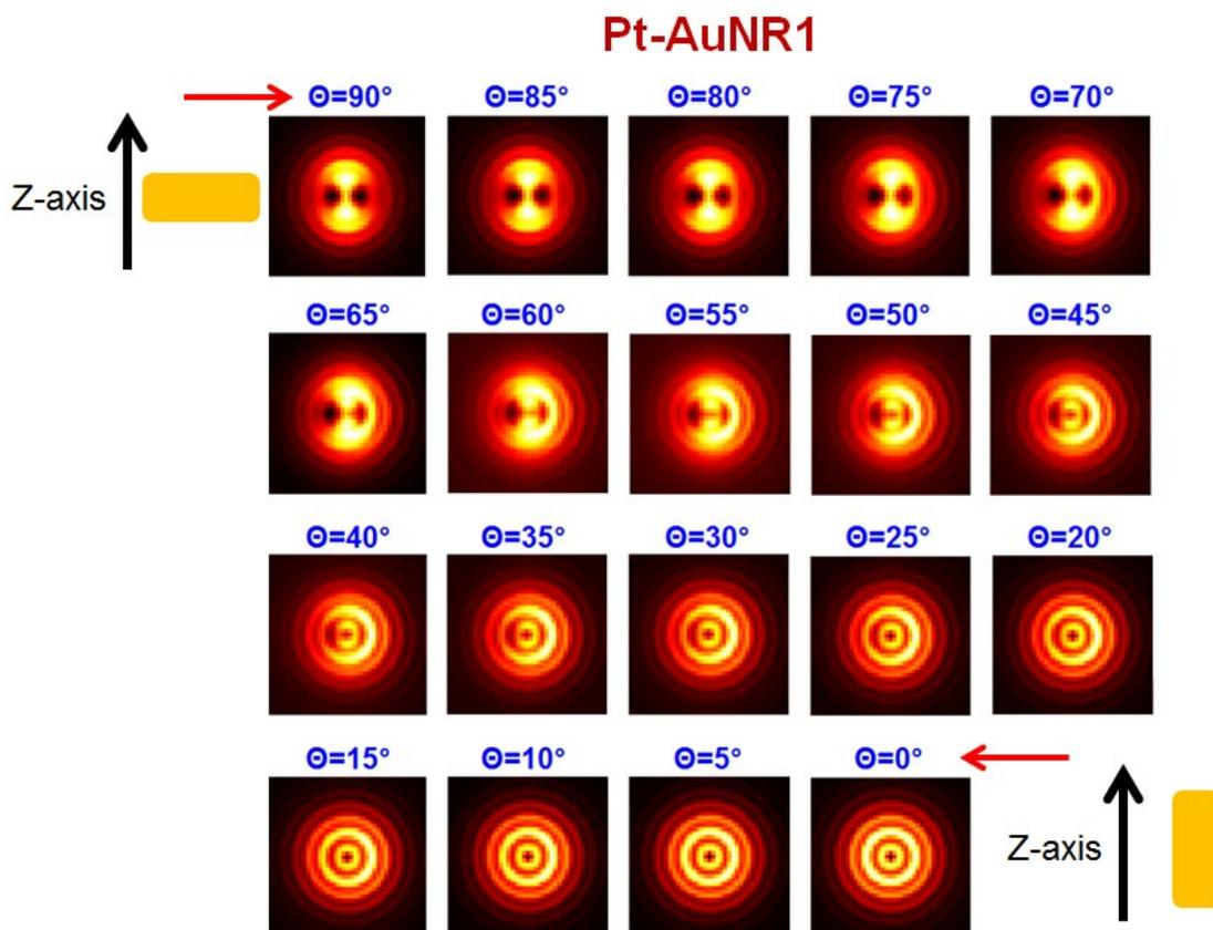
**Fig. S5** The simulated characteristic scattering patterns of a Pt-AuNR by varying the polar angle  $\theta$  from  $0^\circ$  to  $90^\circ$ .
