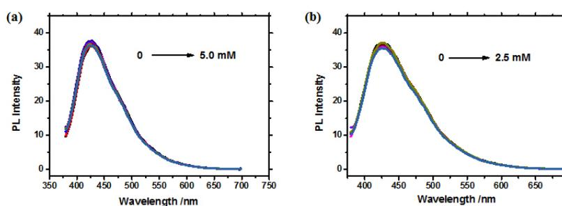
**Fig. S5** The PL intensity evolution of the C-dots when interfering with (a)  $\text{P}_3\text{O}_{10}^{5-}$  up to 5.0 mM, (b)  $\text{SCN}^-$  up to 2.5 mM.
