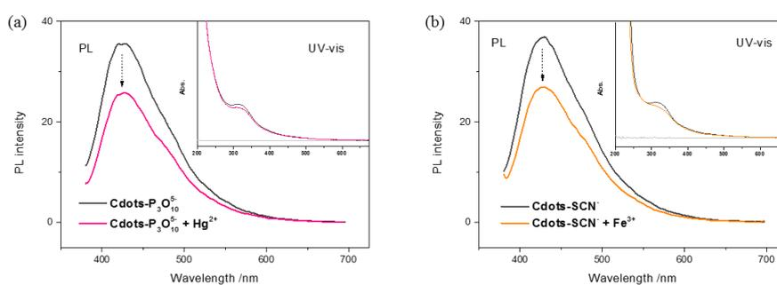
**Fig. S7** PL and UV-vis spectra of the C-dots- $\text{SCN}^-$  and C-dots- $\text{P}_3\text{O}_{10}^{5-}$  system in the absence (black curve) and presence of  $40 \text{ } \mu\text{M}$  (a)  $\text{Hg}^{2+}$  (magenta curve) or (b)  $\text{Fe}^{3+}$  (orange curve), respectively.
