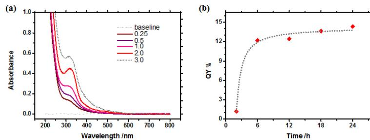
**Fig. S1** (a) The optical absorption evolution of C-dots obtained at various CA/melamine mole ratio and (b) Quantum yields of C-dots as a function of Reaction time.
