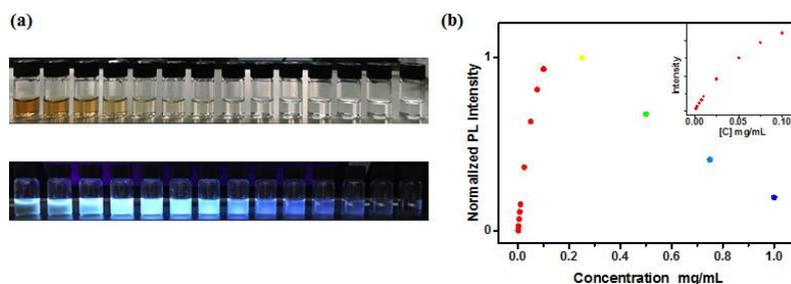
**Fig. S2** (a) Photographs of the C-dots aqueous solution with different concentrations under natural light (top) and 365 nm UV light (down) illumination, and (b) their corresponding PL spectra.
