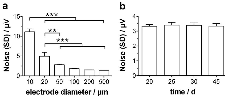
Fig. S4. Characterization of the influence of the electrode diameter on signal noise and long-term stability. **(a)** Analysis of noise standard deviation of recorded field potentials from electrodes with 10 – 500  $\mu\text{m}$  diameter.  $n = 4$  electrodes. **(b)** Analysis of noise standard deviation over prolonged measurement periods (day 20 – 45).
