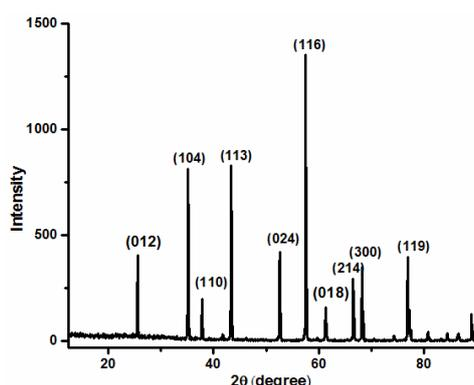
**Fig. 13** XRD pattern of the substrate of Dropsens C110 SPE.
