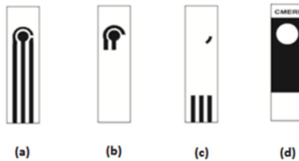
**Fig. 2** Masks involved in the fabrication of SPEs (a) conducting tracking line (b) WE and AE (c) RE and (d) dielectric layer.
