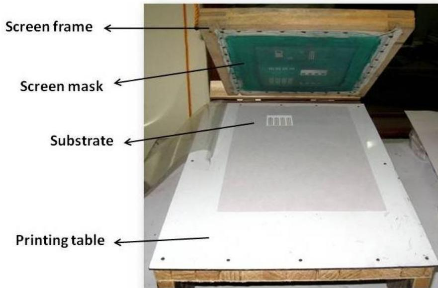
**Fig. 1** Manual screen-printer as set up in laboratory
