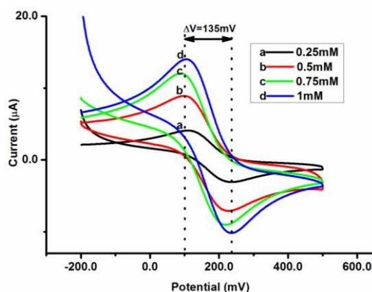
**Fig. 5** CV response of Dropsens C110 SPEs in a set of four different 0.25mM, 0.5mM, 0.76mM and 1mM potassium ferricyanide solution prepared in 0.5M KCl aqueous solution; applied potential scan rate is 50 mV/s.
