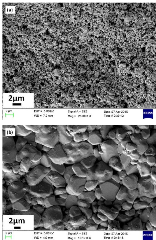
**Fig 8** FESEM of the substrate of (a) laboratory made SPEs and (b) Dropsens C110 SPEs.
