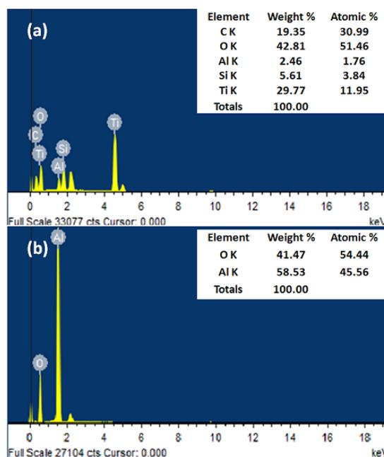
**Fig. 9** EDS of the substrate of (a) laboratory made SPE and (b) Dropsens C110 SPE.
