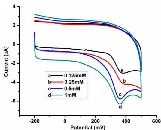
**Fig. 6** CV response of in-house fabricated SPEs in a set of four different 0.125mM, 0.25mM, 0.5mM and 1mM uric acid (UA) solution, prepared in PBS at pH=7; applied potential scan rate is 50 mv/s.
