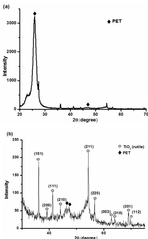
**Fig. 11** XRD pattern of (a) substrate used for fabricating SPE and (b) magnified portion of the same from  $30^\circ$ . (the diamonds represent the phases of PET and the spheres indicate the XRD planes of rutile phase of titania.)
