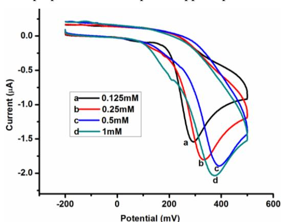
**Fig. 7** CV response of commercial SPE ,Dropsens C110 in a set of four different 0.125mM, 0.25mM, 0.5mM and 1mM uric acid (UA) solution, prepared in PBS at pH=7; applied potential scan rate is 50 mv/s.
