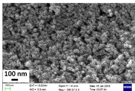
**Fig 10** FESEM of the printed carbon WE of laboratory made SPEs.
