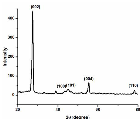
**Fig. 12** XRD pattern of the carbon ink used for fabricating WE and CE of SPE.
