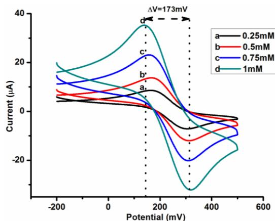
**Fig. 4** CV response of in-house fabricated SPEs in a set of four different 0.25mM, 0.5mM, 0.76mM and 1mM potassium ferricyanide solution prepared in 0.5M KCl aqueous solution; applied potential scan rate is 50 mV/s.
