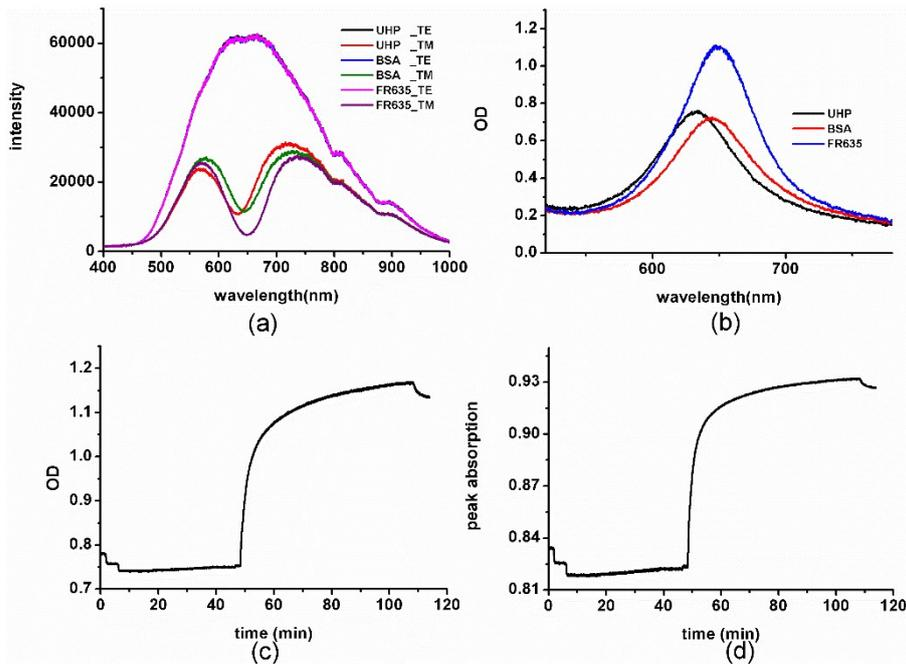
Figure S-2. Peak absorption calculated from optical density(OD). (a) Reflection spectrum with different deposition when illuminated by perpendicular polarization (TE) or parallel polarization (TM); (b) Optical density obtained from (a); (c) Real time OD recording data; (d) Peak absorption calculated from OD.
