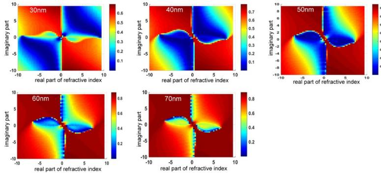
Figure S-1. MI maps based on angular SPR with the excitation wavelength at 633nm for the thickness of gold film is 30nm, 40nm, 50nm, 60nm and 70nm respectively.
