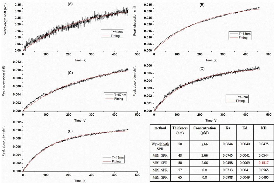
Figure S-3. Sensorgram measured by wavelength and MI SPR methods together with their nonlinear least squares fitting. (A) Wavelength SPR method, gold film thickness=50nm; (B)-(E): MI method, gold film thicknesses are 65nm, 57nm, 50nm, 43nm respectively. The table is the fitting result of each method.
