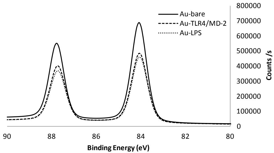
**Fig. S 2** Au 4d XPS signals for bare Au, TLR4/MD-2-modified Au and LPS/TLR4-MD-2-modified Au. The attenuation of these Au 4d signals have been used for estimating the overlayer thicknesses.
