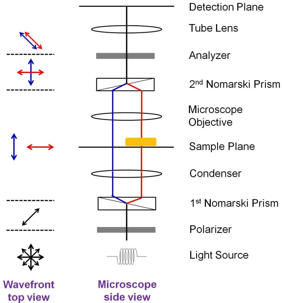
**Fig. S1.** The optical path and wavefront in the DIC microscope. The blue- and red- lines represent the optical path of two orthogonal beams split by the first Nomarski prism.
