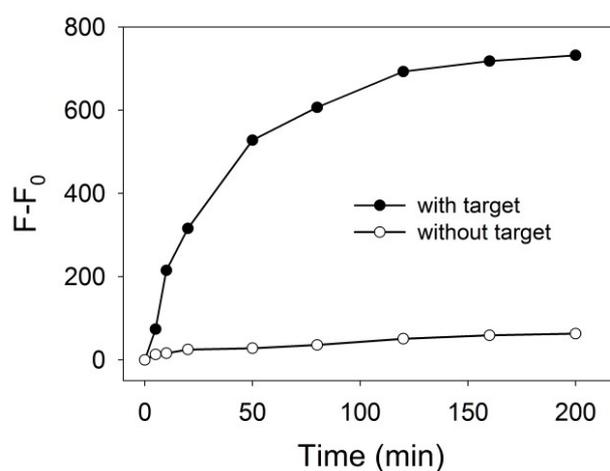
**Fig. S4** Real-time monitoring of the fluorescence intensity in the presence and absence of target DNA ( $\lambda_{ex} = 488$  nm,  $\lambda_{em} = 526$  nm).  $F$  is the fluorescence intensity at the corresponding time point, and  $F_0$  is the fluorescence intensity at the start of the assembly reaction.
