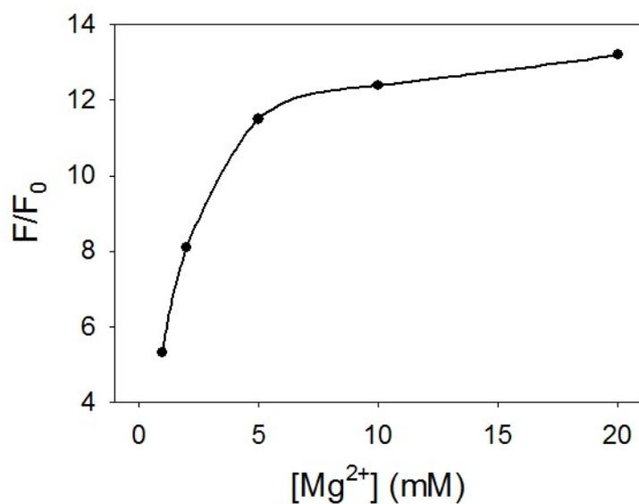
**Fig. S3** The relationship between the fluorescence intensity ratio ( $F/F_0$ ) and the concentration of  $Mg^{2+}$  ions.  $F$  is the fluorescence intensity of FAM in the presence of target DNA, and  $F_0$  is the fluorescence intensity of FAM in the absence of target DNA.  $\lambda_{ex} = 488$  nm,  $\lambda_{em} = 526$  nm.
