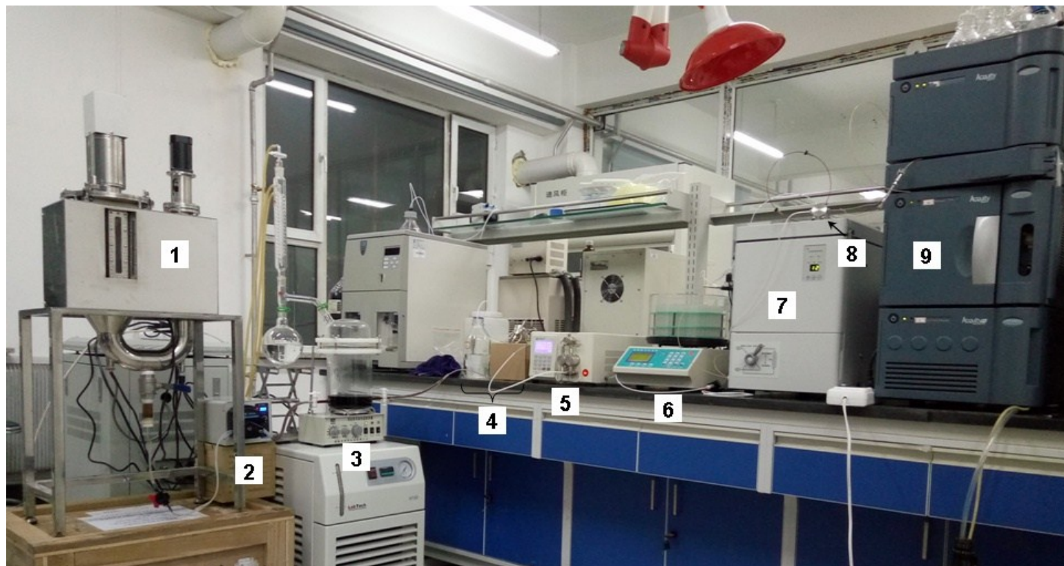
Fig. S1 Photograph of the hyphenation of circulated ultrasound-assisted extraction (CUAE), solvent concentration tank (SCT), centrifugal partition chromatography (CPC), and ultra-high performance liquid chromatography (UPLC)/PDA.
