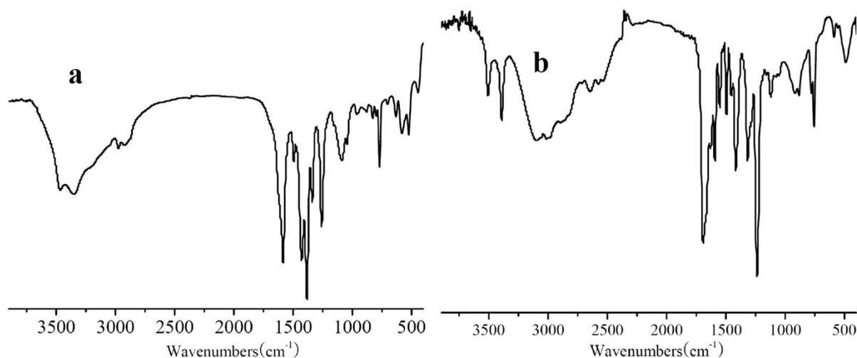
**Figure S4.** FT-IR spectra of the prepared Fe-MIL-88B-NH<sub>2</sub> nanocrystals and used ligand.
