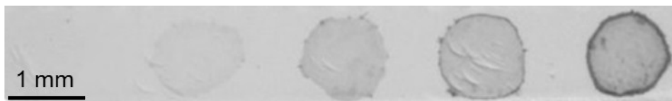
Fig. S8 Optical image of the membrane on which gold nanorods were cast. The image was obtained using light at 680 nm. The membrane was identical to that of Fig. 4 in the main text.
