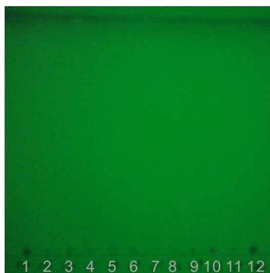
Fig. S3. The TLC image of HDS matrix developed by petroleum ether-acetic ether - acetic acid 5.5:2.8:1(v/v).
