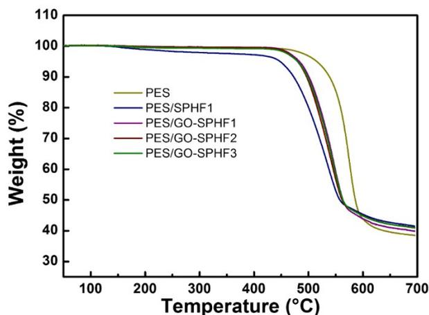
**Figure S3.** The TGA curves for the prepared membranes.
