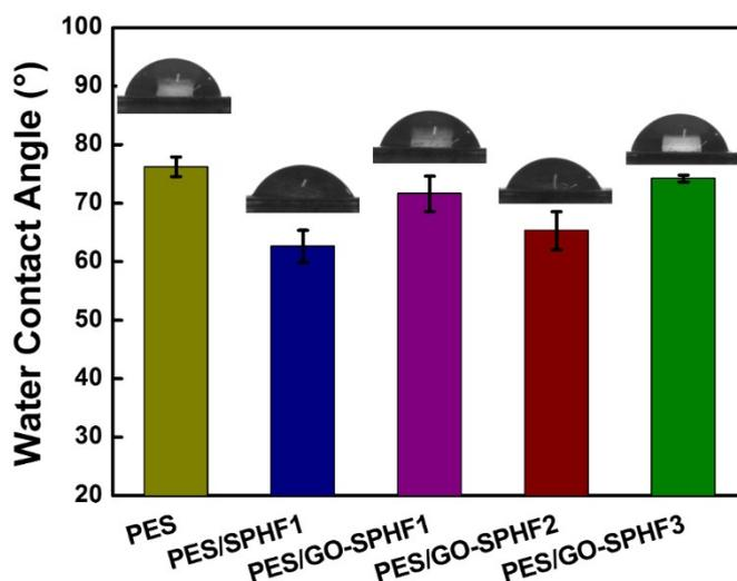
**Figure S4.** The water contact angles of the prepared membranes.
