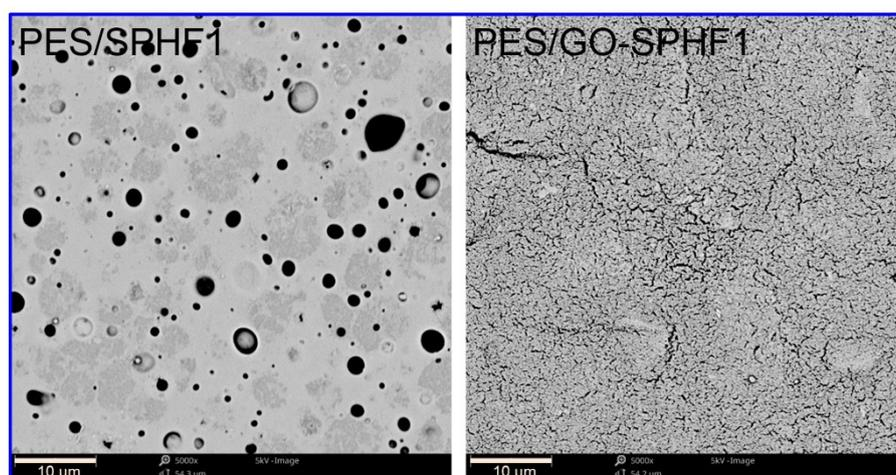
**Figure S2.** Typical surface SEM images of the composite membranes. Voltage: 5.0 kV; magnification: 5000× with the scale bar of 10 μm.
