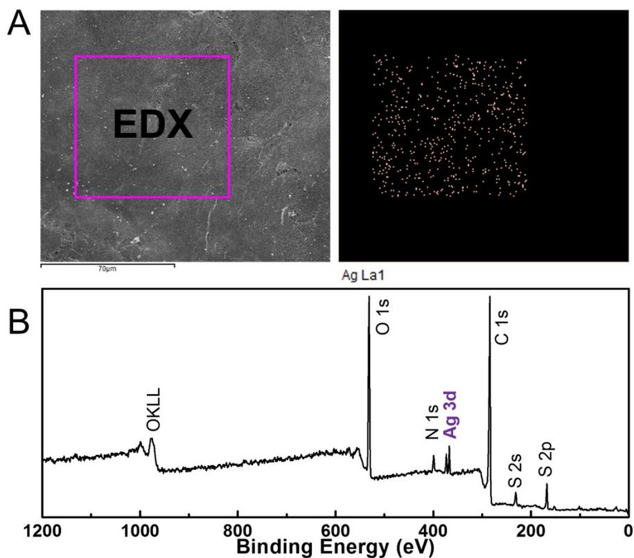
**Figure S6.** (A) EDX mapping analysis of the Ag-nanoparticles loaded membrane PES/GO-SPHF3-Ag. (B) XPS spectrum of the Ag-nanoparticles loaded membrane PES/GO-SPHF3-Ag.
