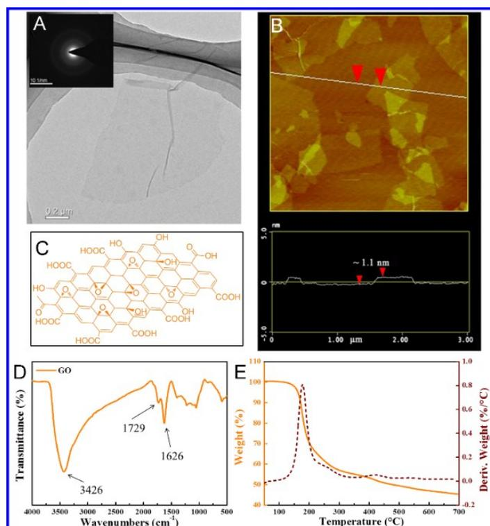
**Figure S1.** (A) TEM image and corresponding SAED patterns of GO. (B) Typical AFM image and cross-section analyse of GO. (C) Chemical structure of GO. (D) FTIR spectrum for the prepared GO. (E) The TGA image for the prepared GO.
