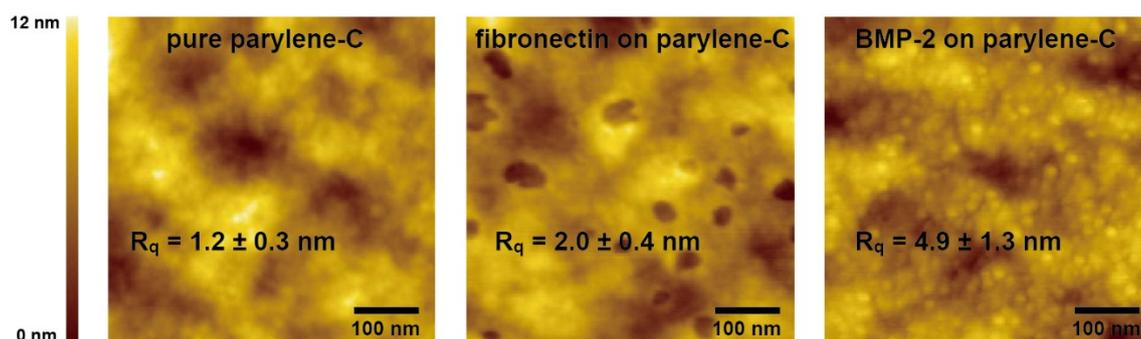
**Figure S2.** Surface roughness analysis by AFM for pure parylene-C surface, adsorption of fibronectin on parylene-C and adsorption of BMP-2 on parylene-C. The root-mean-square roughness ( $R_q$ ) of  $1.2 \pm 0.3$  nm,  $2.0 \pm 0.4$  nm and  $4.9 \pm 1.3$  nm was measured for parylene-C, fibronectin and BMP-2, respectively.
