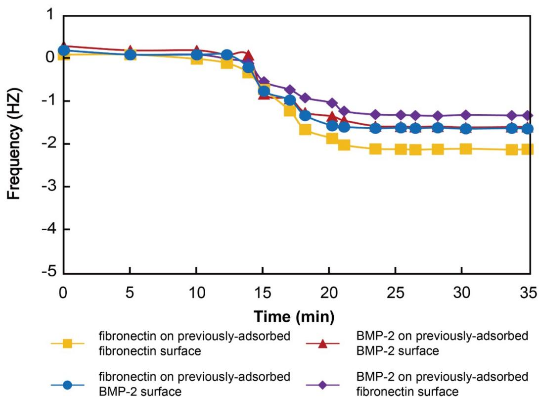
**Figure S3.** QCM analysis of adsorption stability by introducing secondary BMP-2 or fibronectin proteins to the first adsorption surfaces of BMP-2 or fibronectin. Low frequency changes were detected irrespective to the protein types on the adsorption surfaces of BMP-2 and fibronectin.
