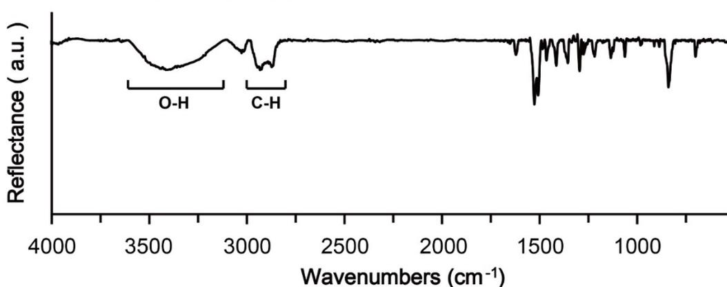
**Figure S1.** IRRAS spectra of PEG-modified surface. The characteristic bond *O-H* ( $3200\text{-}3600 \text{ cm}^{-1}$ ) were detected, indicating the presence of PEG on PEG-modified surface.
