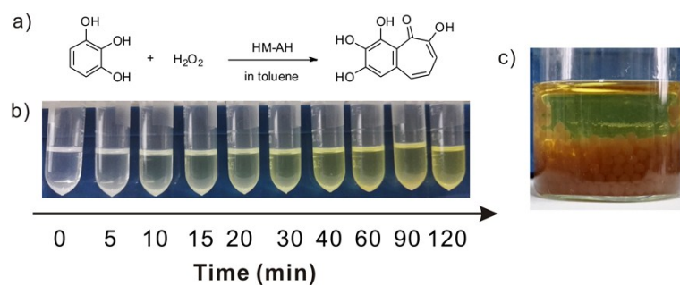
Fig. S15 (a) The peroxidized model reaction catalyzed by HM-AH in toluene. (b) Color changes of the substrates pyrogallol in toluene along with the catalytic reactions. (c) The optical image of HM-AH in toluene during the catalytic reaction.
