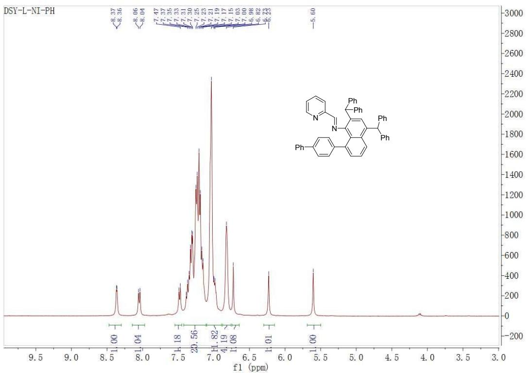
**Figure S15.**  $^1\text{H}$  NMR spectrum of L3 in  $\text{CDCl}_3$ .
