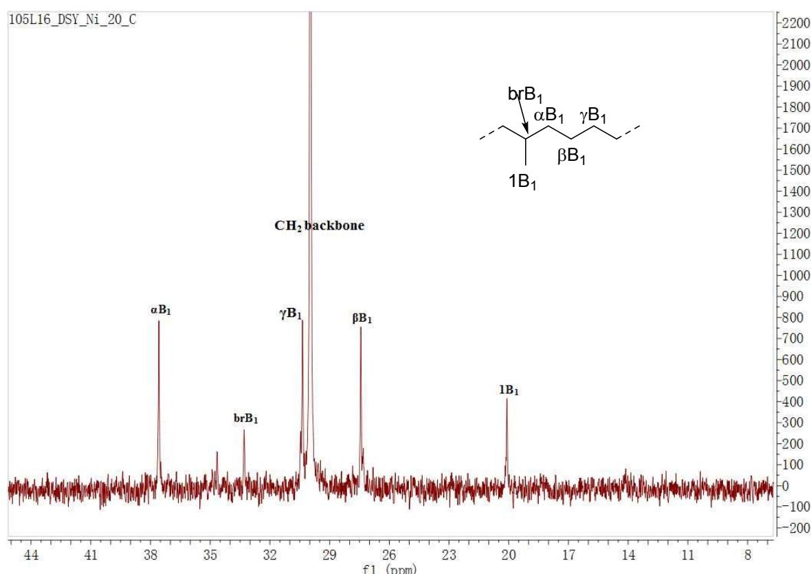
**Figure S22.** <sup>13</sup>C NMR spectrum of the polymer from table 1, entry 1.
