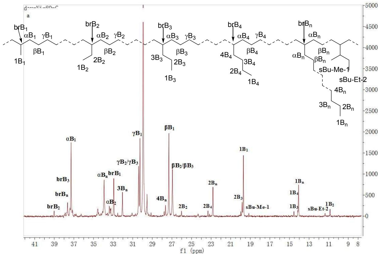
Figure S24.  $^{13}\text{C}$  NMR spectrum of the polymer from table 1, entry 3.
