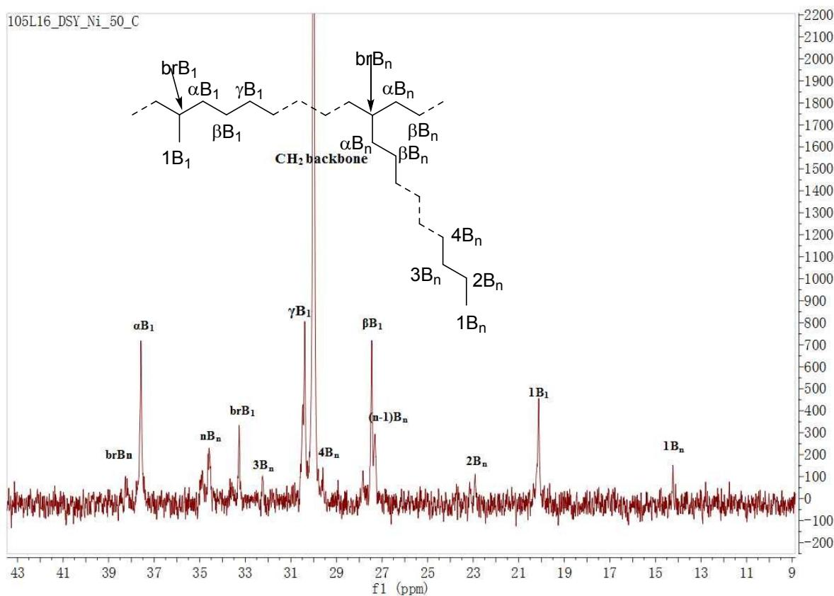
Figure S23.  $^{13}\text{C}$  NMR spectrum of the polymer from table 1, entry 2.
