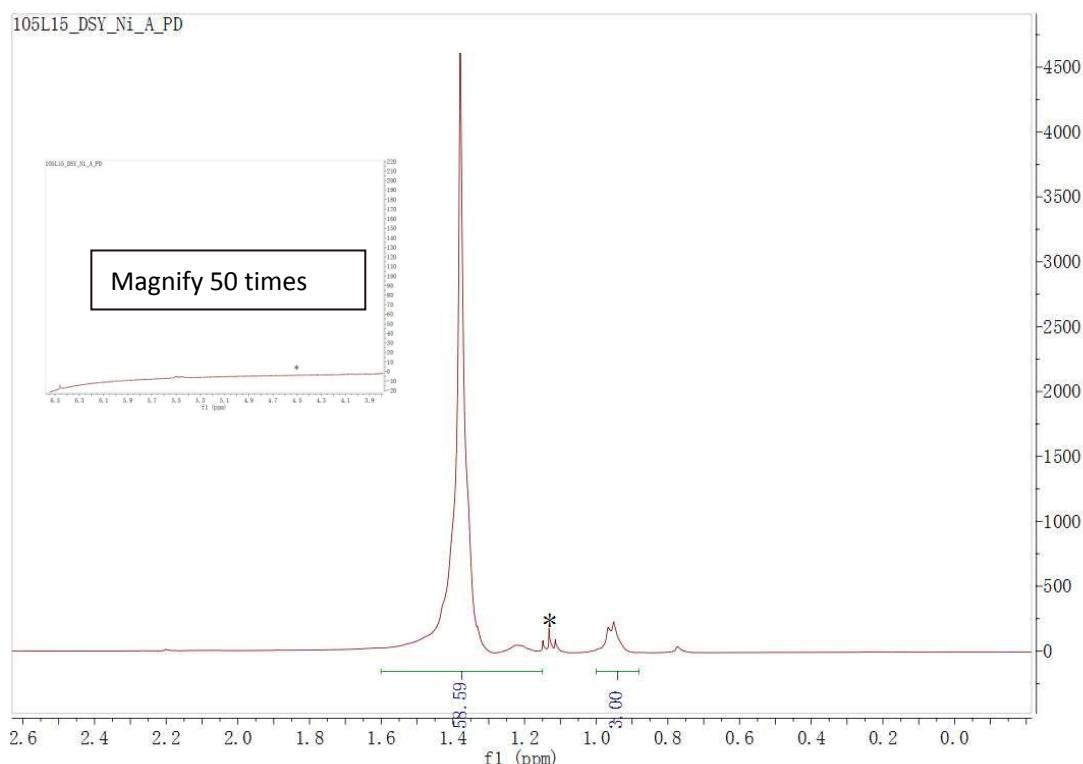
**Figure S26.** <sup>1</sup>H NMR spectrum of the polymer from table 2, entry 4. \*CH<sub>3</sub>CH<sub>2</sub>OH (d<sup>6</sup>-benzene:1,2,4-trichlorobenzene=1:3 (v/v) 100°C).
