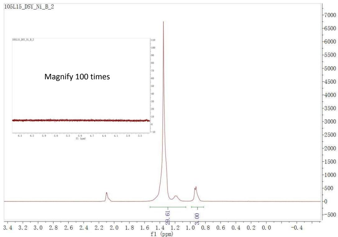
**Figure S20.**  $^1\text{H}$  NMR spectrum of the polymer from table 1, entry 6 (Insert: the region of  $\delta$  6.0–4.0, magnify 100 times). ( $d^8$ -toluene, 80°C).
