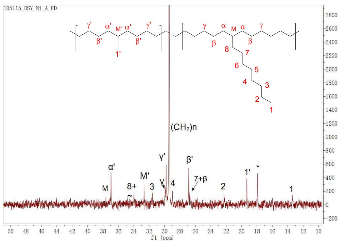
**Figure S27.**  $^{13}\text{C}$  NMR spectrum of the polymer from table 2, entry 4.  $^*\text{CH}_3\text{CH}_2\text{OH}$  ( $\text{d}^6\text{-benzene:1,2,4-trichlorobenzene=1:3 (v/v) } 100^\circ\text{C}$ ).
