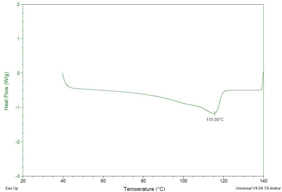
**Figure S30. DSC of the polymer from table 1, entry 7**
