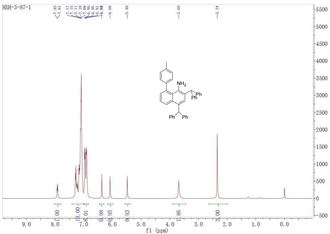
**Figure S5.**  $^1\text{H}$  NMR spectrum of S7 in  $\text{CDCl}_3$ .
