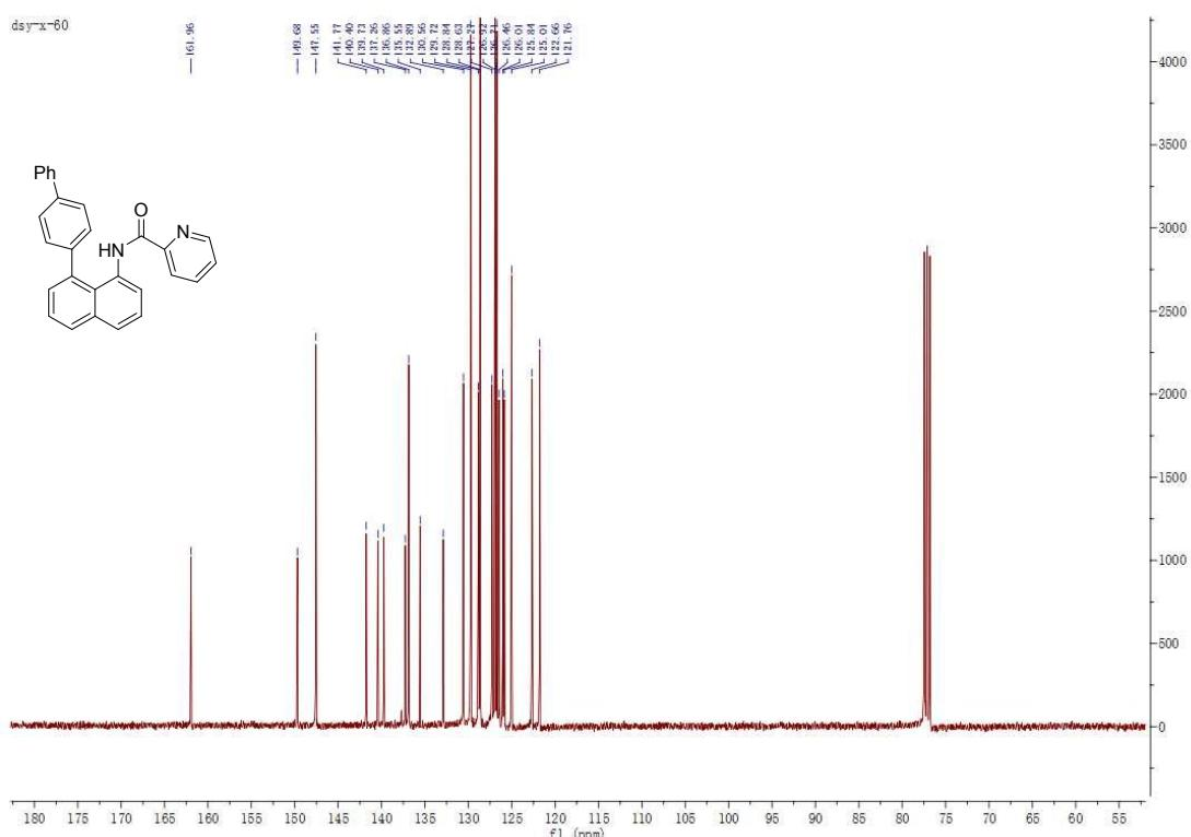
**Figure S2.**  $^{13}\text{C}$  NMR spectrum of S3 in  $\text{CDCl}_3$ .
