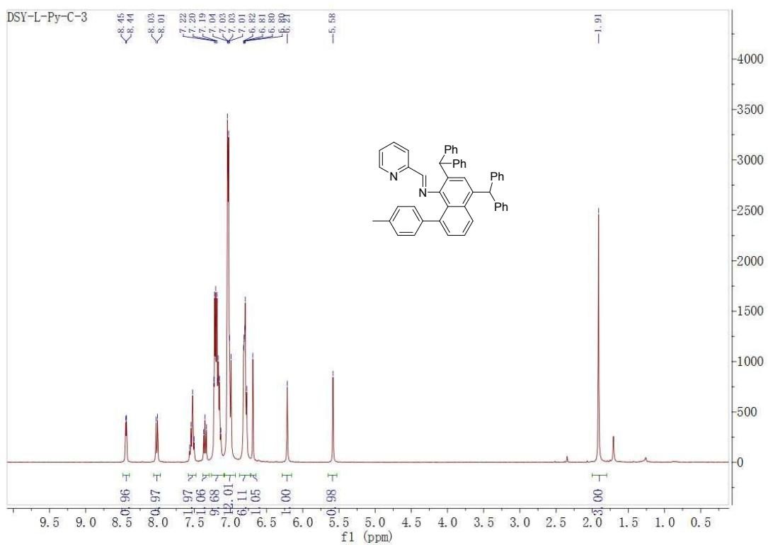
**Figure S11.**  $^1\text{H}$  NMR spectrum of L1 in  $\text{CDCl}_3$ .
